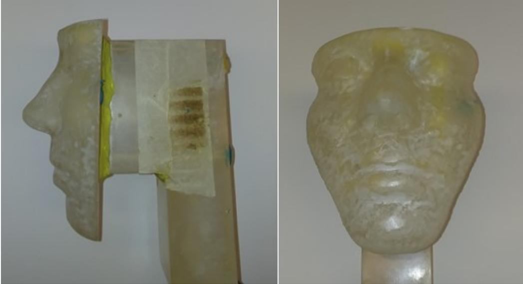
*Figure 2-1: Side and front view of upper airway replica. Specific replica shown corresponds to "Subject 2".*
