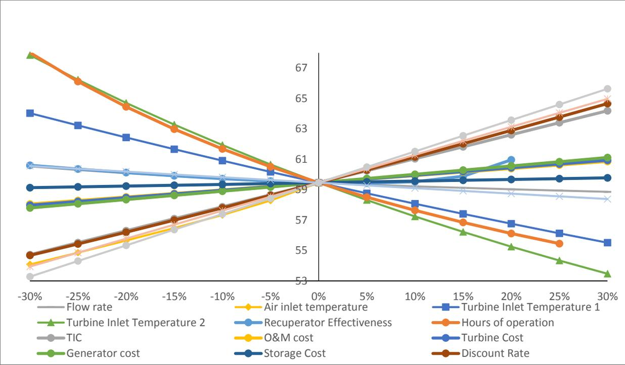
Figure 19: Effect of variations of different parameters on the levelised cost of electricity for conventional compressed air energy storage
