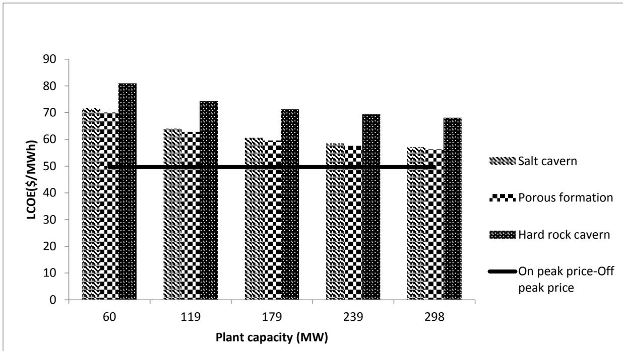
Figure 17: Variations of levelised cost of storage with plant capacity for adiabatic compressed air energy storage
