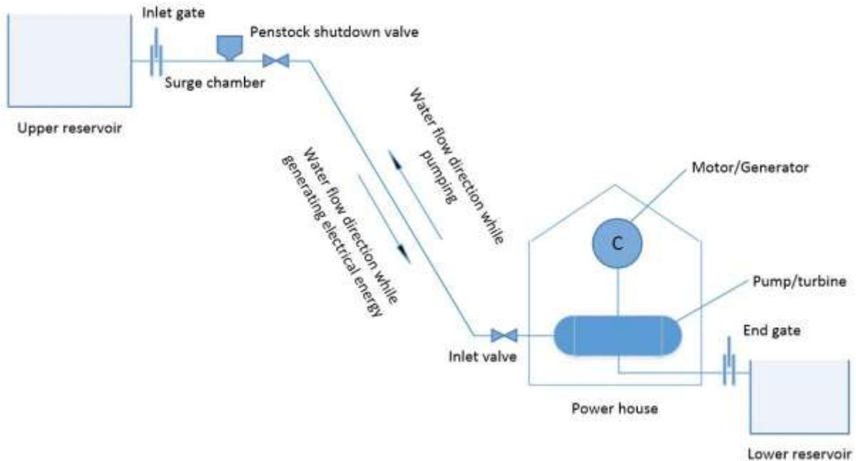
Figure 2: Pumped hydro storage schematic
