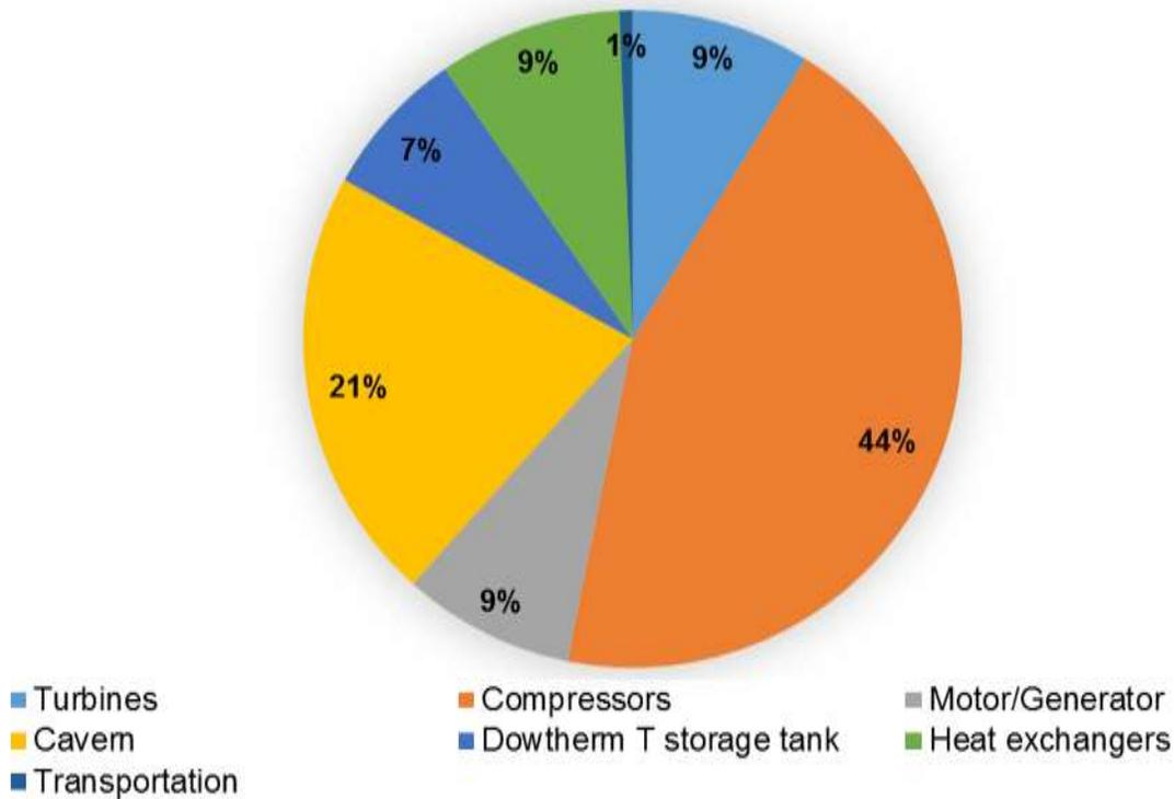
Figure 32: Breakdown of construction emissions for A-CAES
