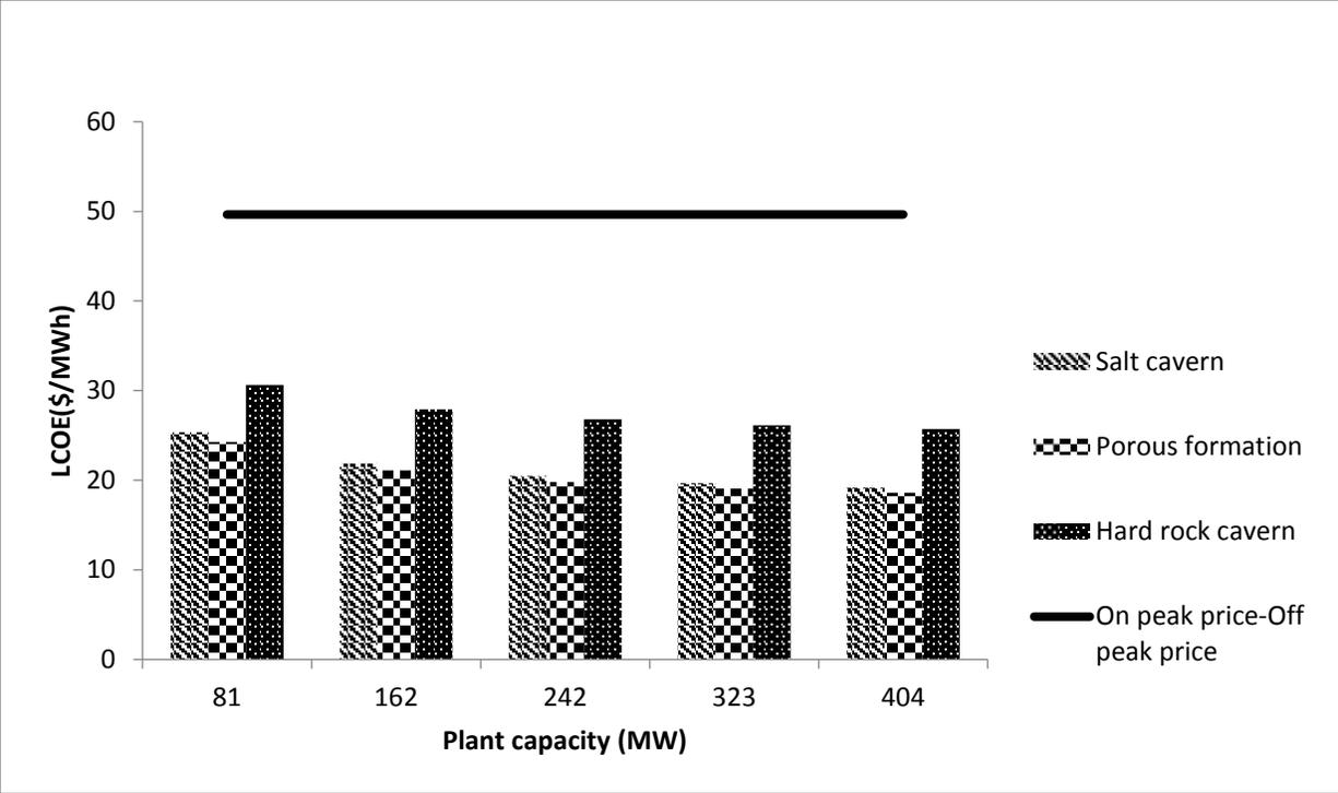
Figure 16: Variations of levelised cost of storage with plant capacity for conventional compressed air energy storage
