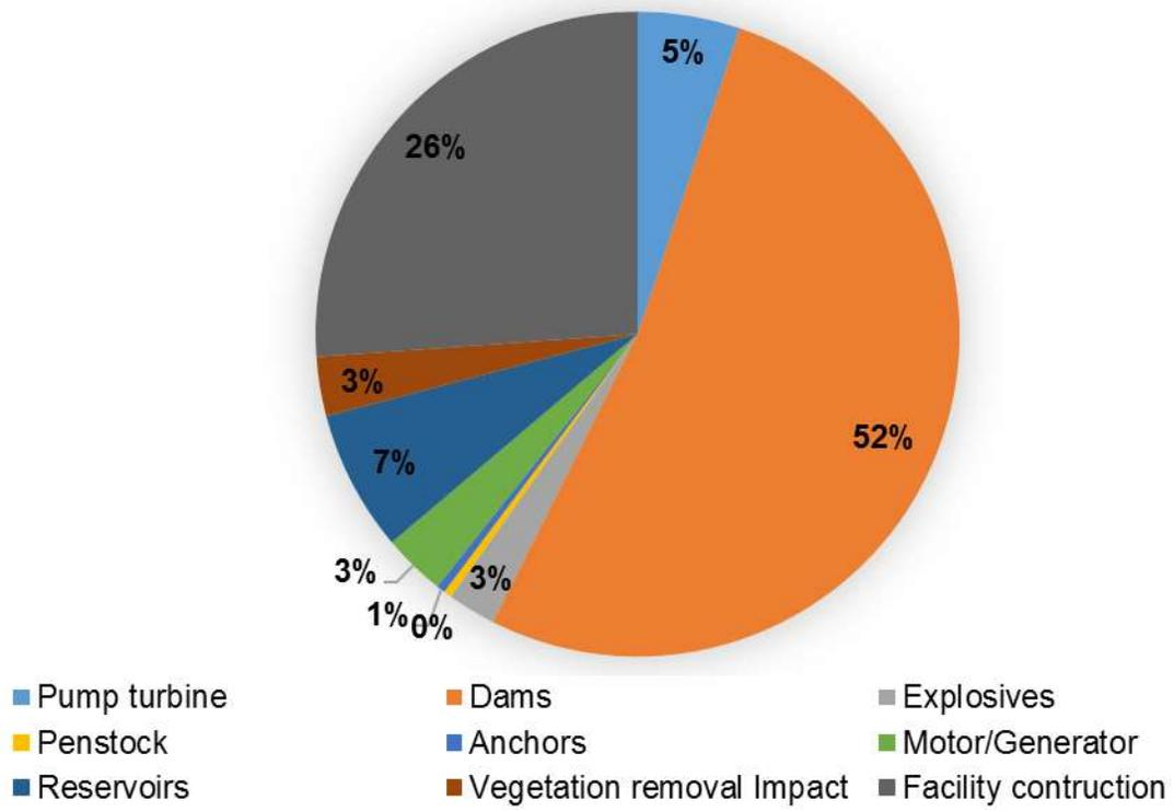
Figure 30: Breakdown of construction emissions for PHS
