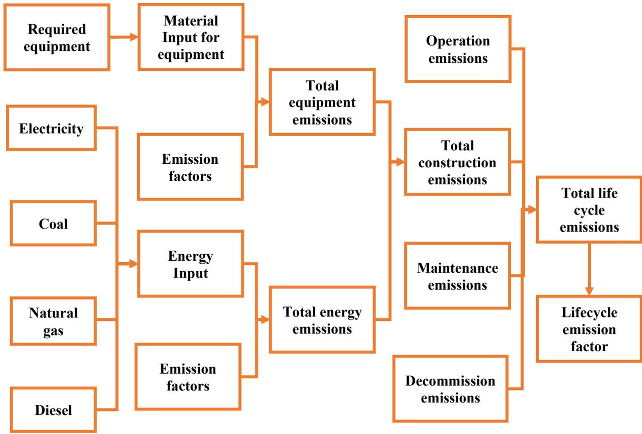
Figure 26: LCA system boundary
