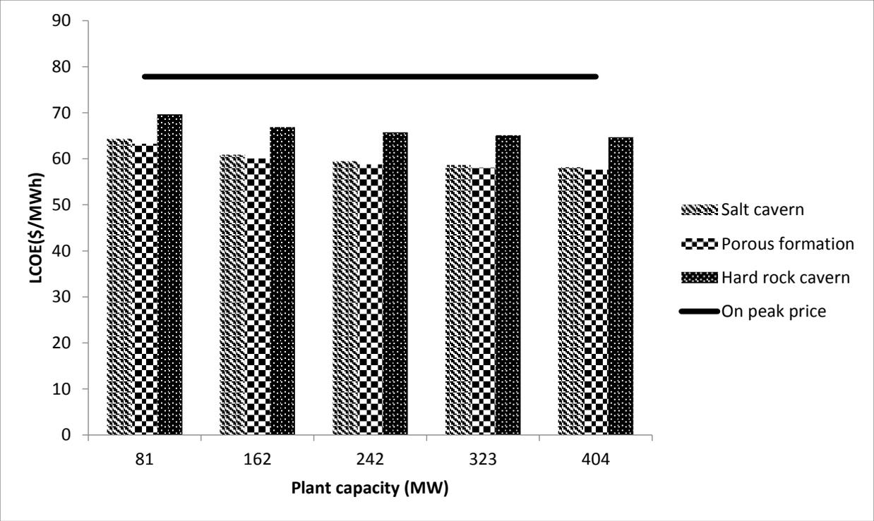
Figure 13: Variations of levelised cost of electricity with plant capacity for conventional compressed air energy storage
