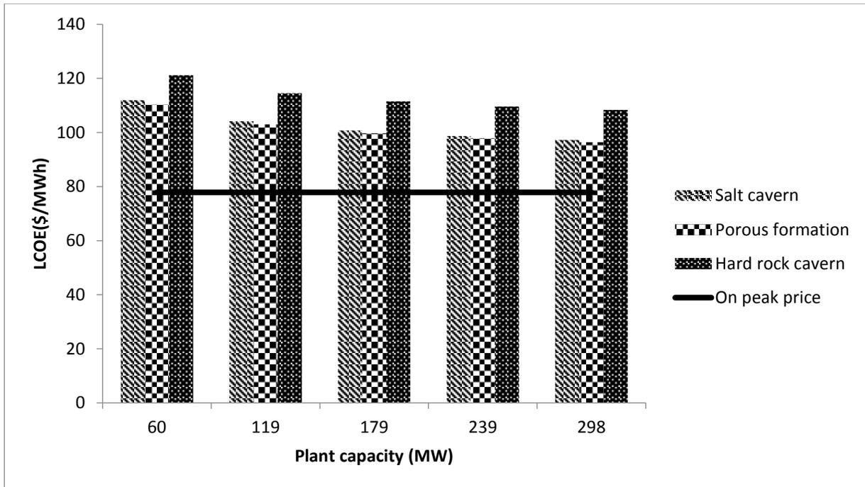
Figure 14: Variations of levelised cost of electricity with plant capacity for adiabatic compressed air energy storage
