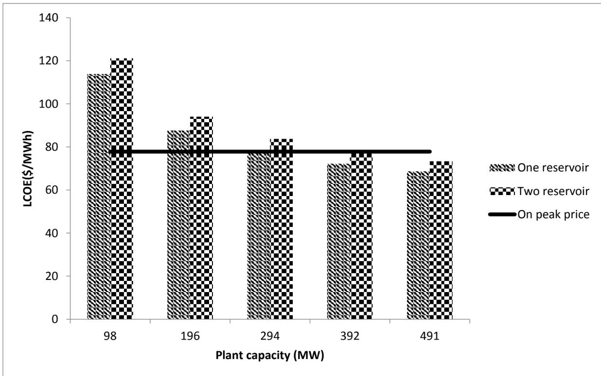
Figure 12: Variations of the levelised cost of electricity with plant capacity for pumped hydro storage
