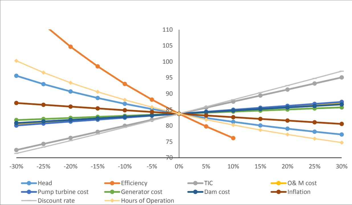
Figure 18: Effect of variations of different parameters on the levelised cost of electricity for pumped hydro storage
