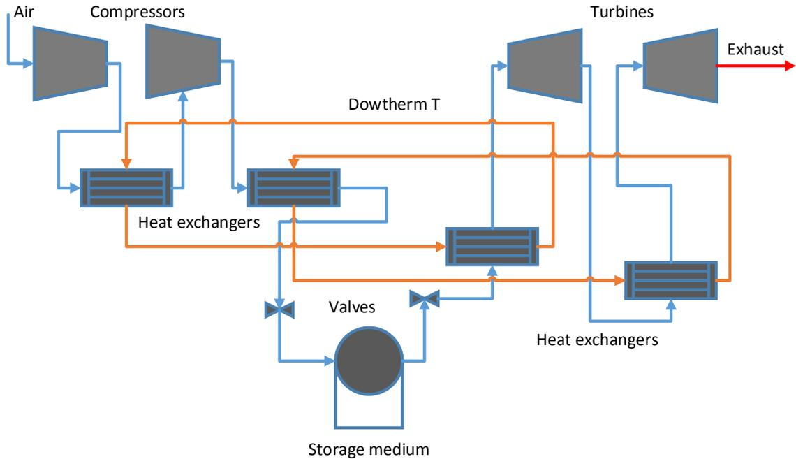
Figure 24: Adiabatic compressed air energy storage system diagram
