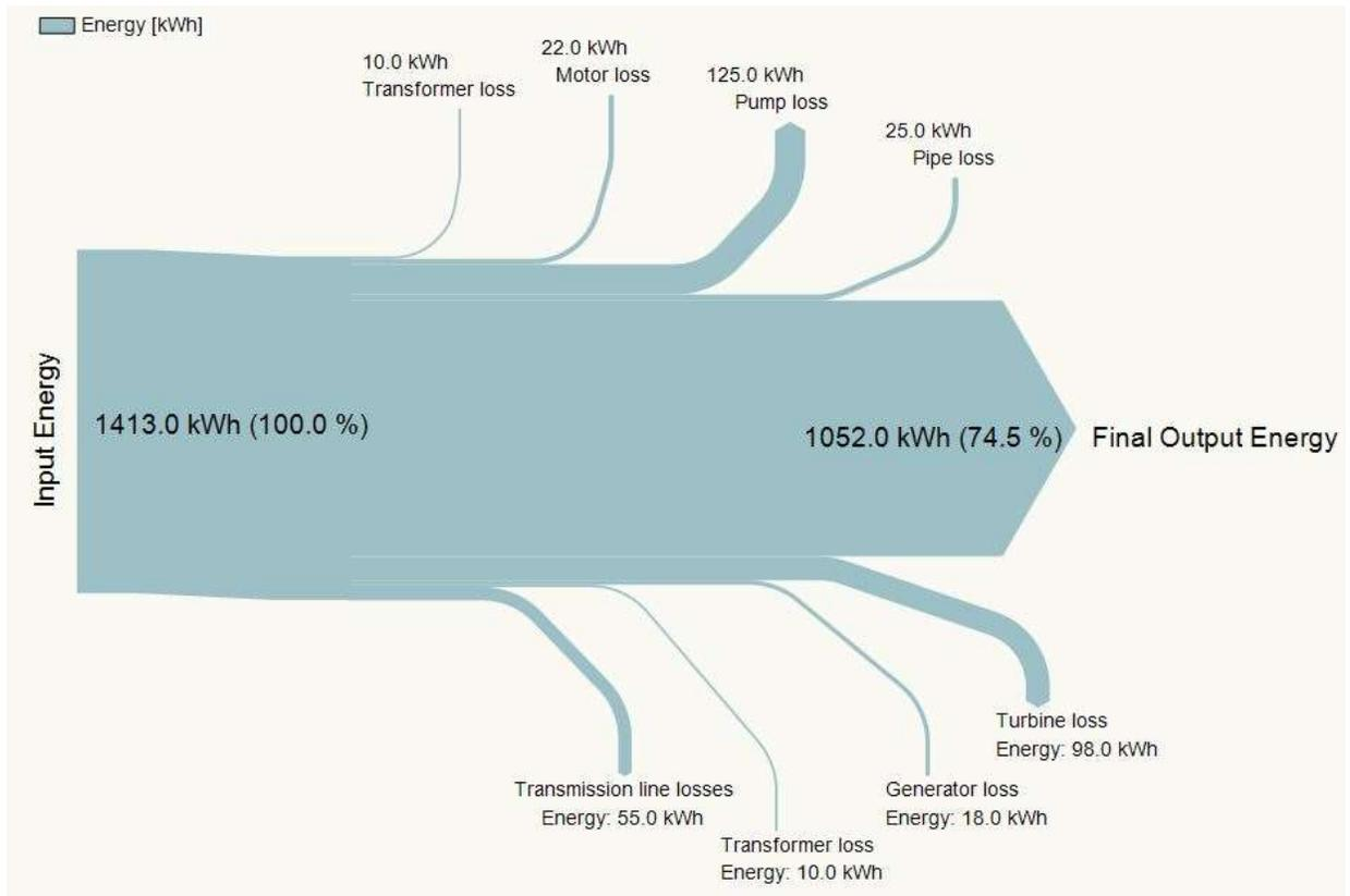
Figure 27: Energy flow diagram for single PHS cycle
