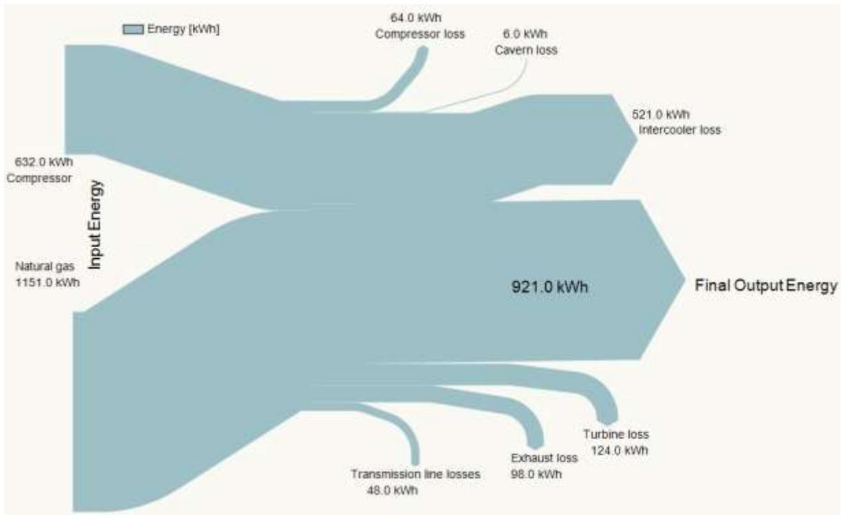
Figure 28: Energy flow diagram for single C-CAES cycle
