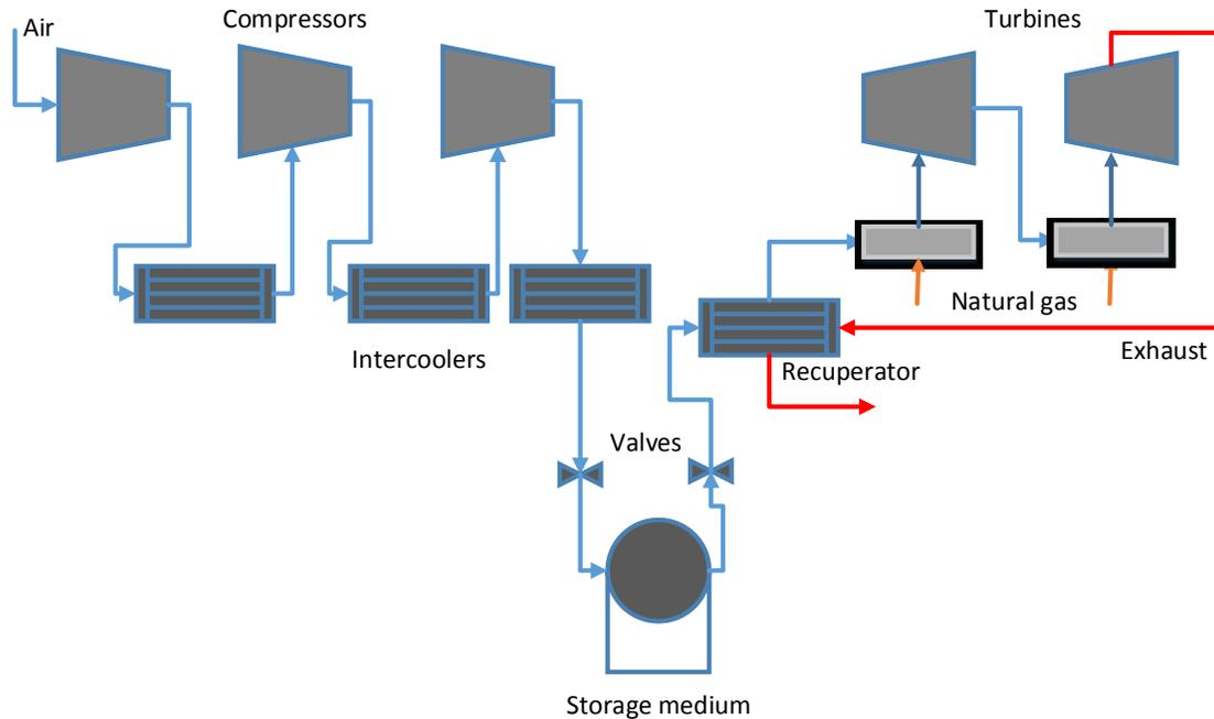
Figure 23: Conventional compressed air energy storage system diagram
