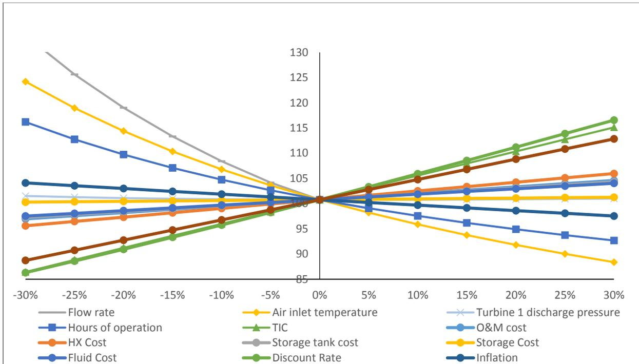
Figure 20: Effect of variations of different parameters on the levelised cost of electricity for adiabatic compressed air energy storage
