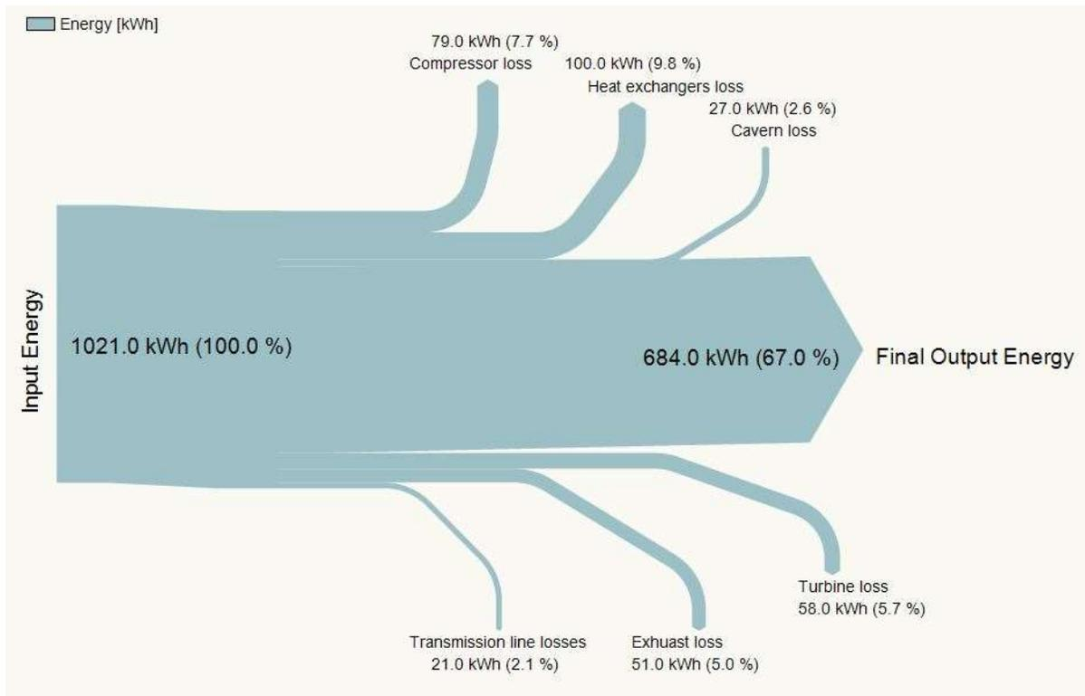
Figure 29: Energy flow diagram for single A-CAES cycle
