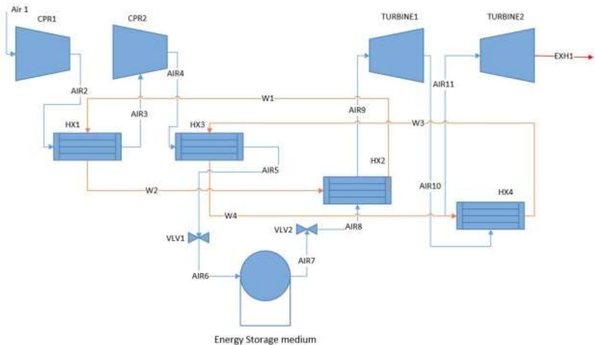
Figure 4: Adiabatic compressed air energy storage schematic
