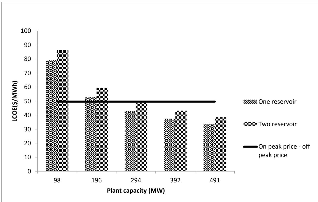
Figure 15: Variations of levelised cost of storage with plant capacity for pumped hydro storage
