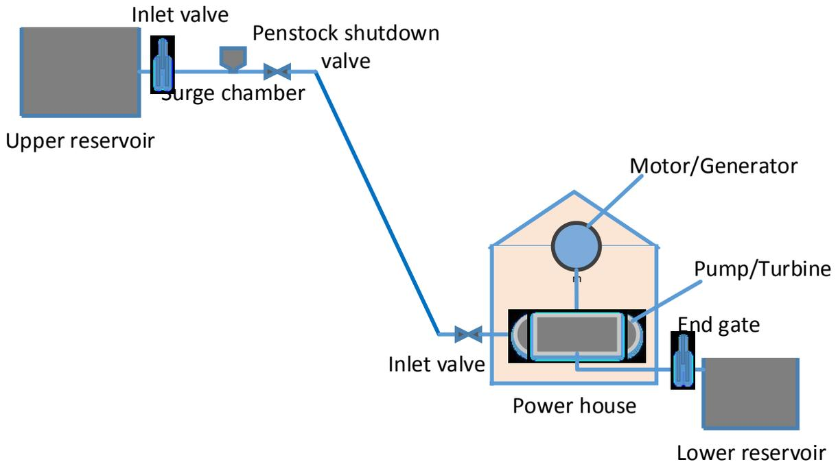
Figure 22: Pumped hydro storage system diagram
