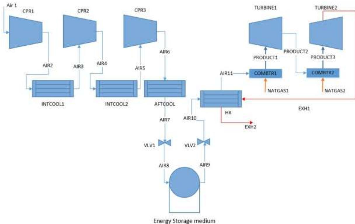
Figure 3: Conventional compressed air energy storage schematic
