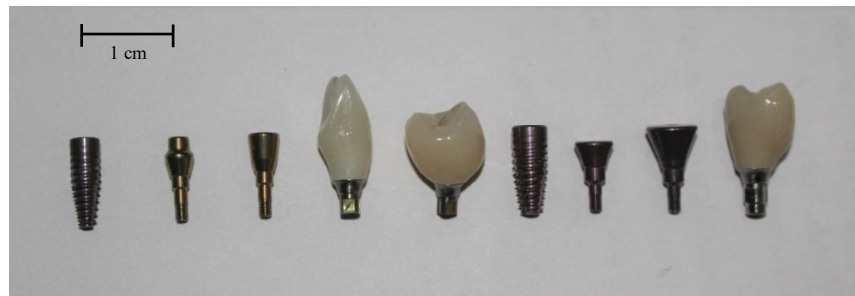
Figure 3.1: Implants, abutments, and crowns. From left to right: NC implant, 3.3HA, 3.6HA, IN, NCP, RC implant, 4.5HA, 6.0HA, RCP.
