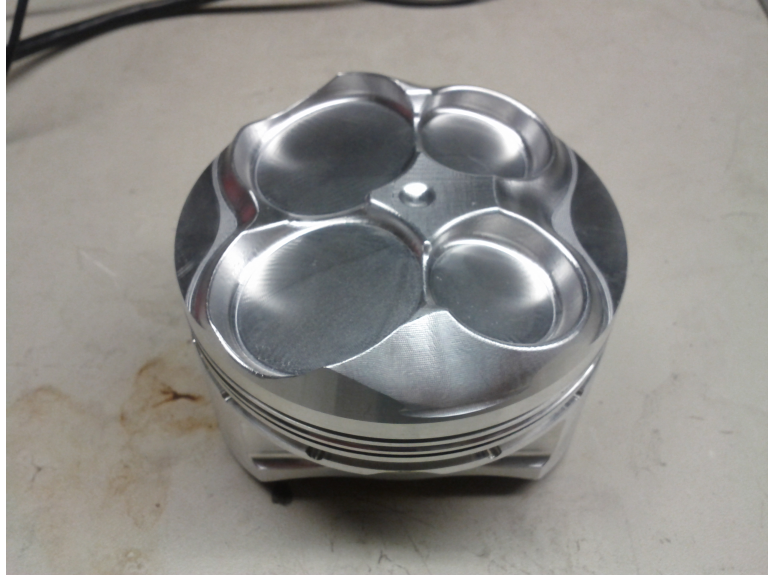
Figure 3.1: 97mm diameter piston crown used with the EVVT valves.
