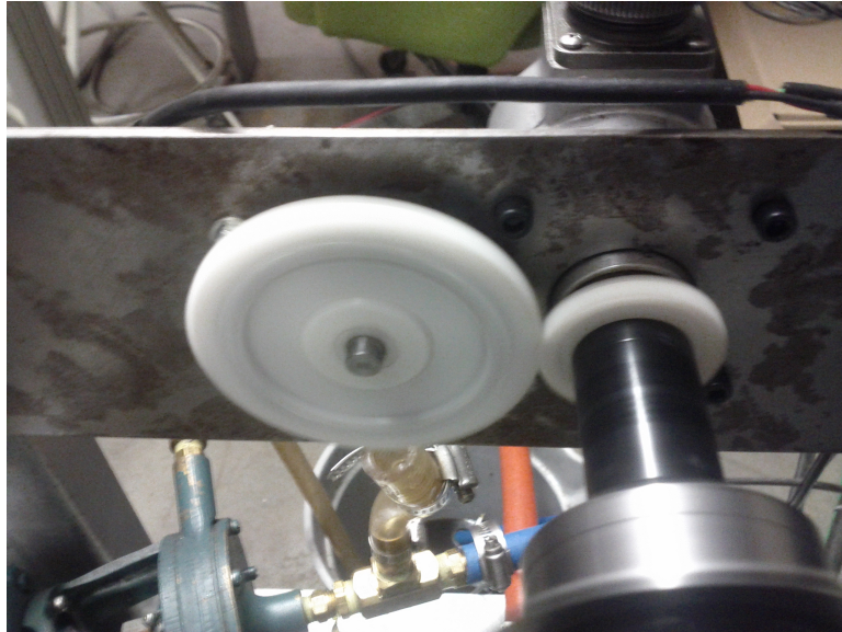
Figure 3.5: Photograph of the cam encoder gear setup.
