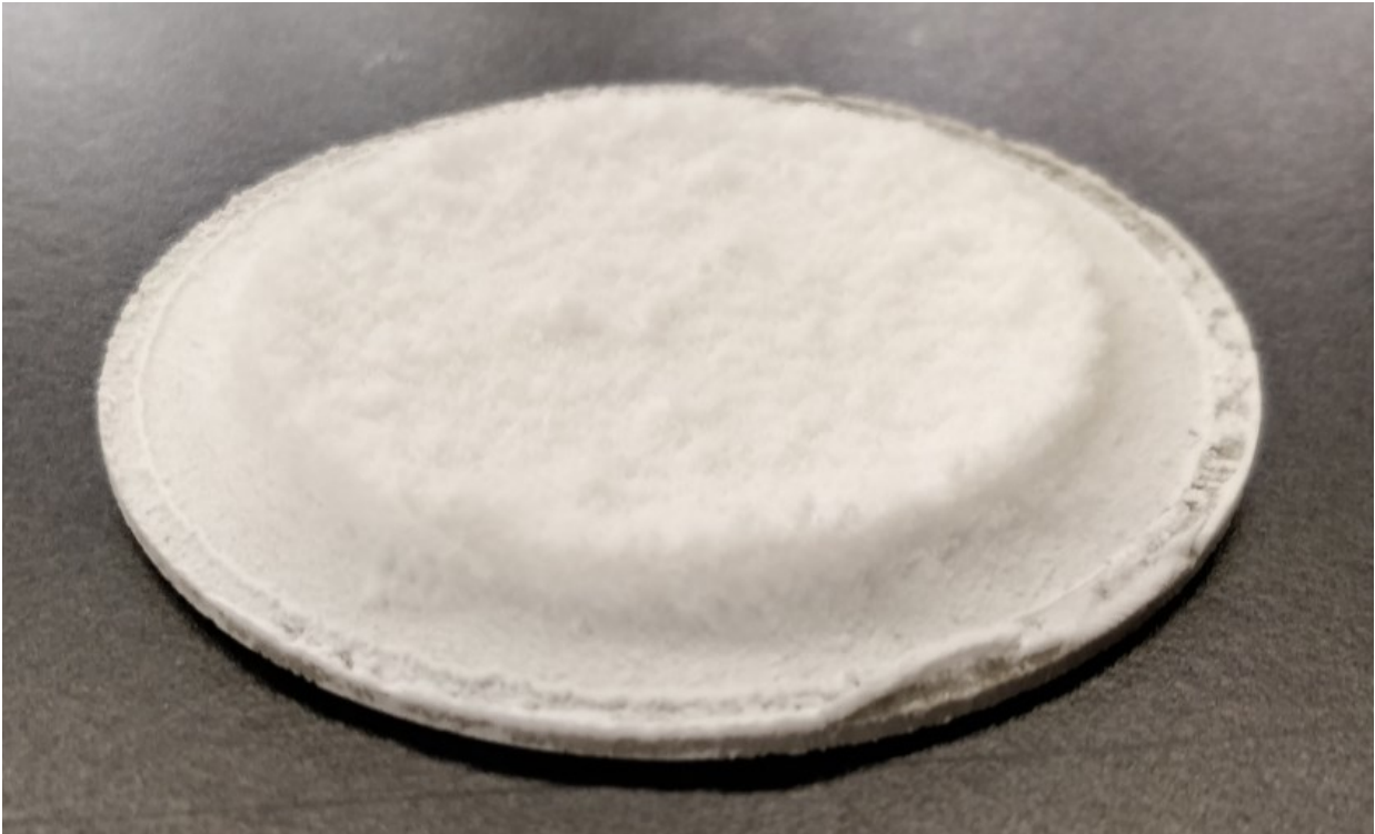
Figure 2.3 ASFD trehalose powder at feedstock concentration of 100 mg/mL after removing from ASFD apparatus
