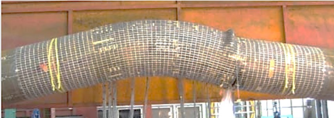
Figure 2-14: Rupture of pressurized cold bend pipe on tensile side of the wrinkled location under opening curvature ( Mitsuya et al. 2008)
