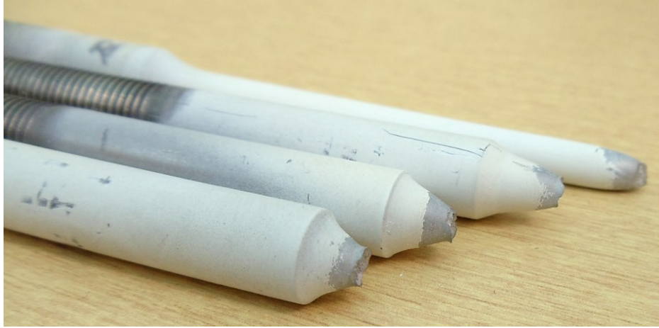
Figure 4-12: Failure mode of RB specimens
