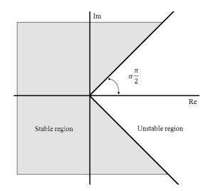
Figure 2.1: Stability region of fractional order LTI system (2.15) with order  $0 < \alpha < 1$ .
