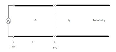
Figure 3.2: Infinite length transmission line.
