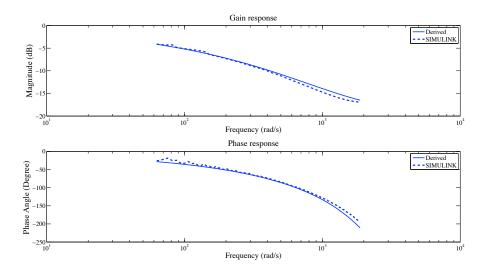
Figure 4.2: Comparison of the Bode plots of semi-infinite length or terminated line with matched load.
