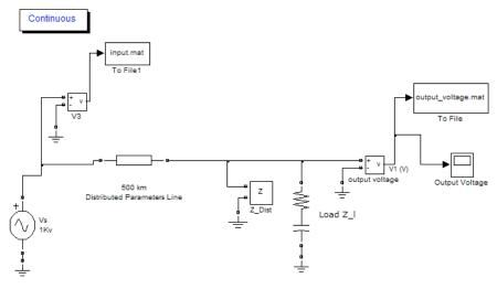
Single Phase Line - Time and Frequency Domain Testing
