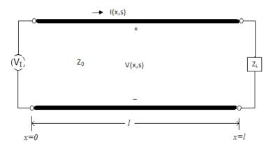
Figure 3.4: A lossy transmission line terminated by a load impedance  $Z_L$ .
