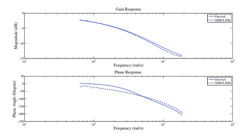
Figure 4.3: Comparison of the Bode plots of finite length line terminated with load  $2Z_0(s)$ .
