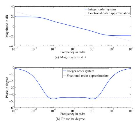
Figure 1.1: Comparison between a high order integer system and its approximation by fractional one.
