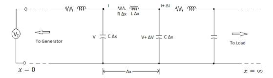
Figure 3.1: Circuit representation of uniform transmission line.
