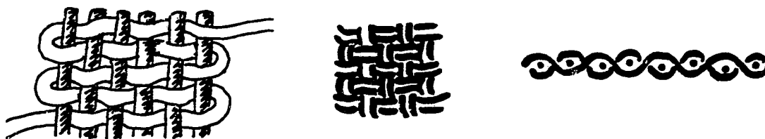
Figure 38. Various representations of plain weave structure (Sketches by J.A. Renzi, 1995).
