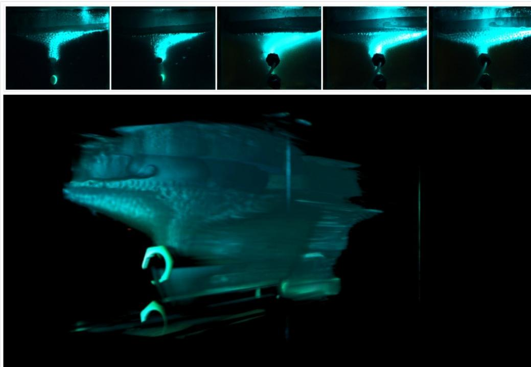
**Fig. 3.30—VAPEx injected at 1.5 ml/min into the model with low permeability zone at the top at 1 cm, 5 cm, 10 cm, 15 cm, 17.5 cm and 3-D images from the heel at 147 min.**
