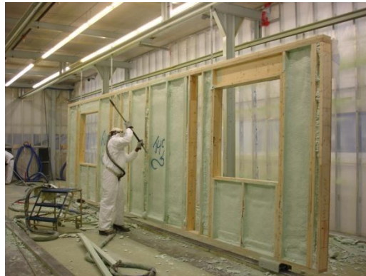
Station W8: Spray foam insulation booth
