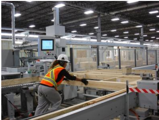
Station W2: Framing table
