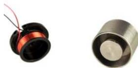
Figure 1.9: Small physical size of coil sensor.
