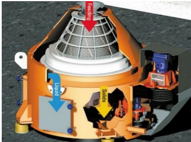
Figure 1-14 A vertical cuttings dryer can process drill cuttings up to 60 tons per treatment and achieve ~ 5 wt% ROC. Reprinted with permission from Ref 17 [17]. Copyright © 2019 M.-I. SWACO.
