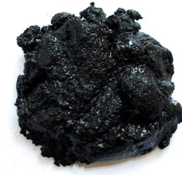
Figure 1-5 Picture of drill cuttings used in this thesis. The drill cuttings were contaminated by the oil-based drilling fluids.
