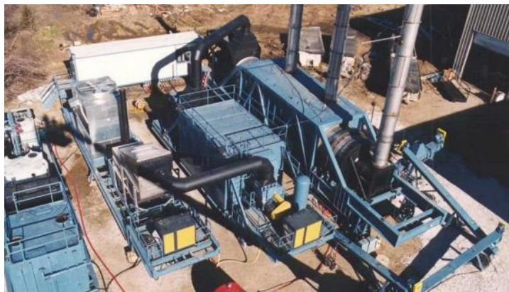
Figure 1-15 Pictures of typical thermal desorption stations for the oil-contaminated drill cuttings treatment. Reprinted with permission from Ref 21 [21]. Copyright © 2002 Society of Petroleum Engineers.
