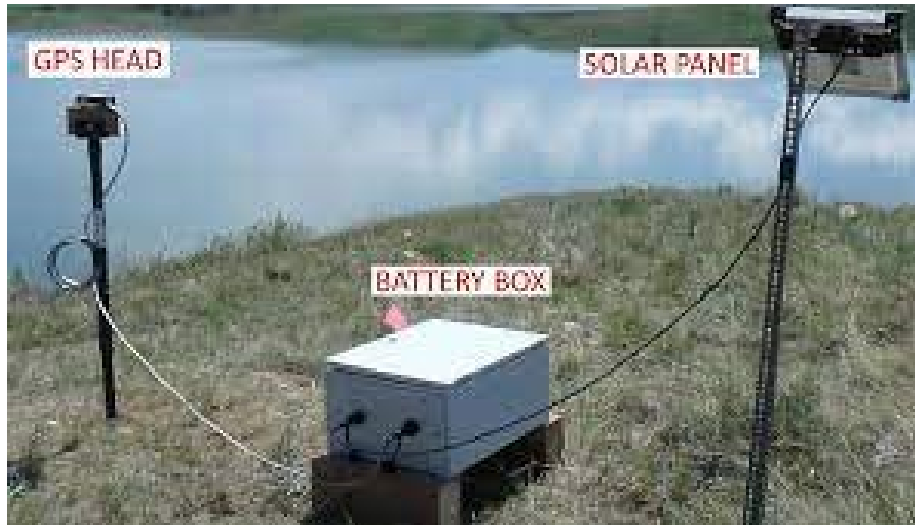
Figure 37:GPS and Battery Box Setup on Chin Coulee (Deane E. et al. 2019)
