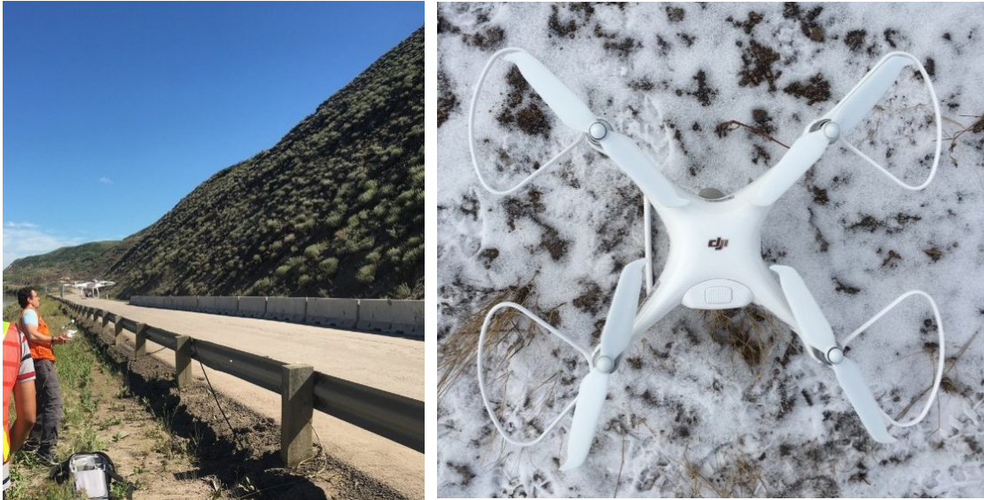
Figure 20: UAV/Drone DJI Phantom 4 with 12 MP camera and 3-axis stabilizer used for CO18 site.
