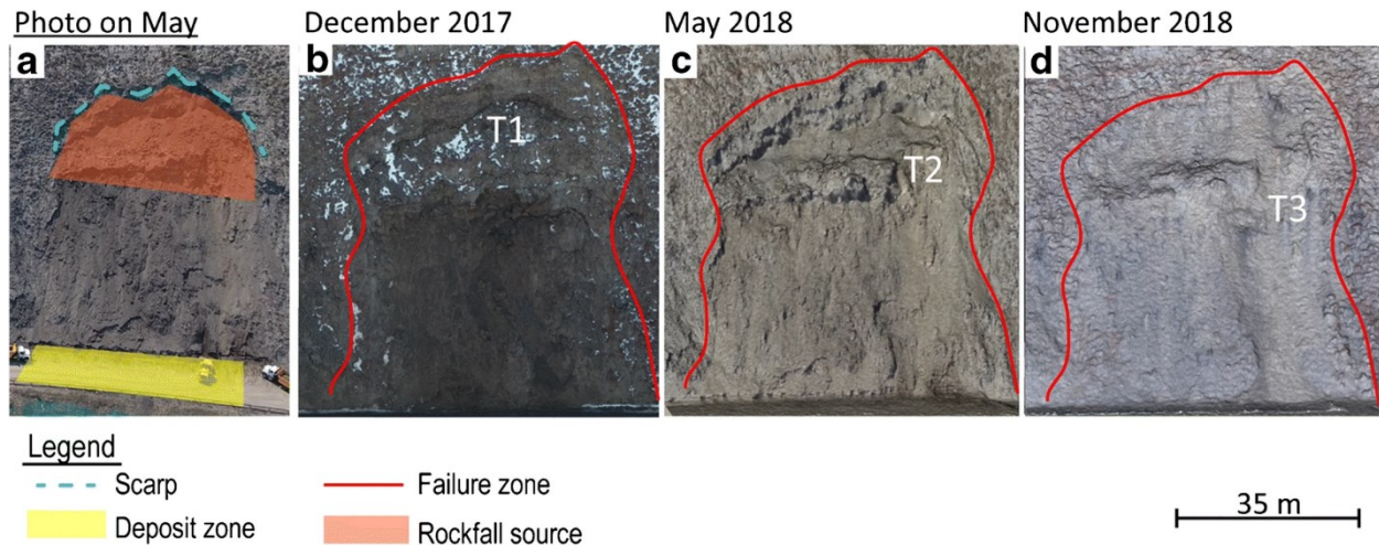
Figure 44: Point clouds for the most active zone a) UAV photo taken after May event b) point cloud from first UAV survey c) from second UAV survey d) from third UAV survey (Rodriguez et al. 2020 licensed under CC BY 4.0 )
