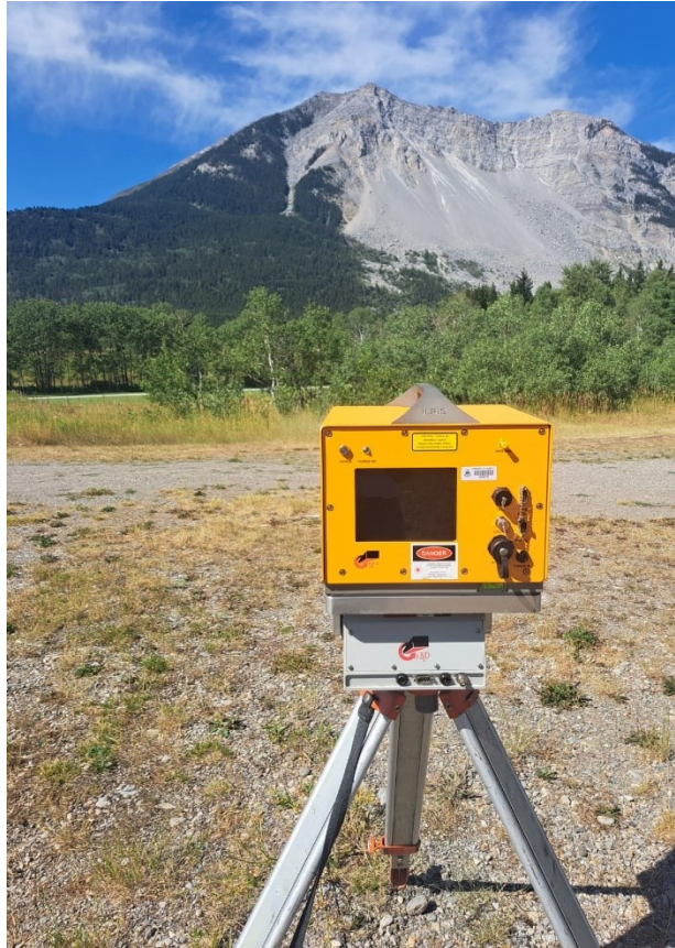
Figure 19: Use of TLS LiDAR at Frank Slide in Southern Alberta
