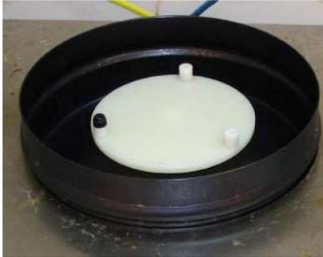
**Figure C -2 Image of the Teflon wafer holder in the bowl.**
