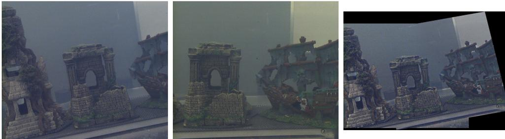
(C) Photos taken after adding milk (level 2) and the stitching result using dehazing.
