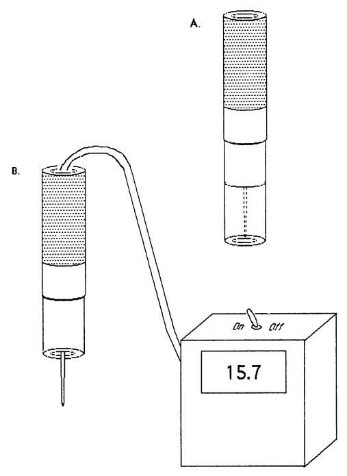
Figure 5-1. The h-gun, used for taking quantitative wood hardness measurements from snag, log, and stump wood sections. Wood hardness measurements are inversely proportional
