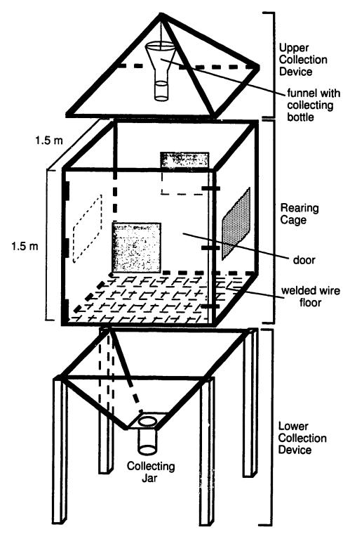
Figure 2-1. Cage design for rearing of arthropods from coarse woody material.
