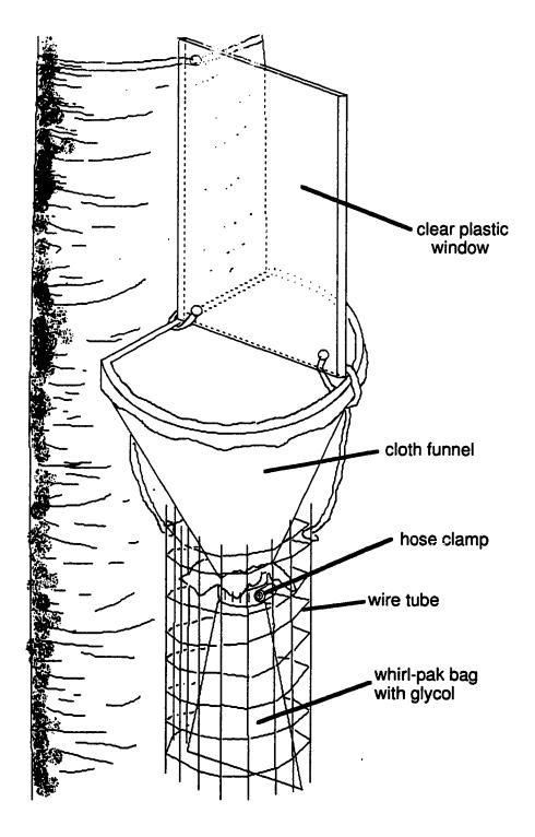
Figure 2-2. Window-trap design (modified from Kaila, 1993) for sampling arthropods associated with coarse woody material.
