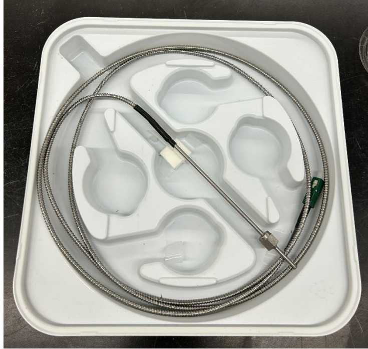
FIG 2-1 Fiber optic pressure sensor
