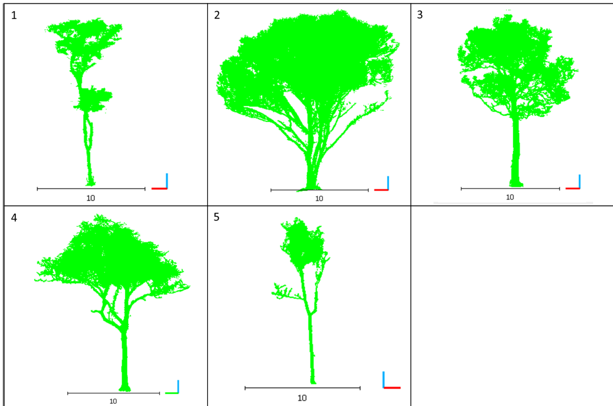
Figure 3.1: Forested trees merged point-clouds with a spatial resolution of 0.01 meter. Tree colours represent the same living environment since the species was not gathered. Forested individuals were dominant emergent trees. The scale below each tree measures 10 meters.
