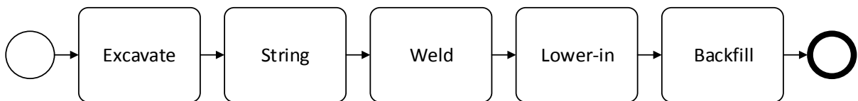
Figure 4.6: Pipeline Construction Tasks
