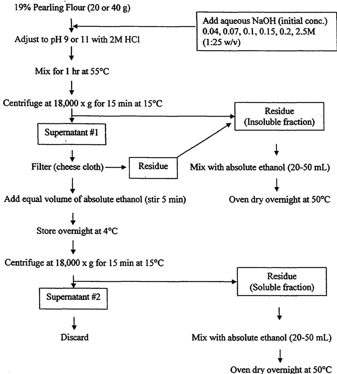
**Figure 3.1.** Flow diagram for the recovery of soluble and insoluble fractions from 19% pearling flour of CDC Candle barley at different initial alkali concentrations and pH.
