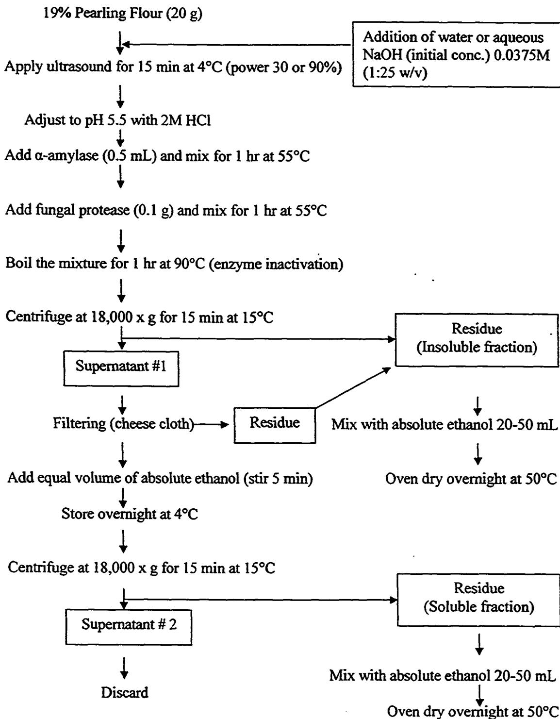
**Figure 4.2.** Flow diagram for the recovery of soluble and insoluble fractions from 19% pearling flour of CDC Candle barley in water or 0.0375M NaOH using combined ultrasound and enzymatic treatments.
