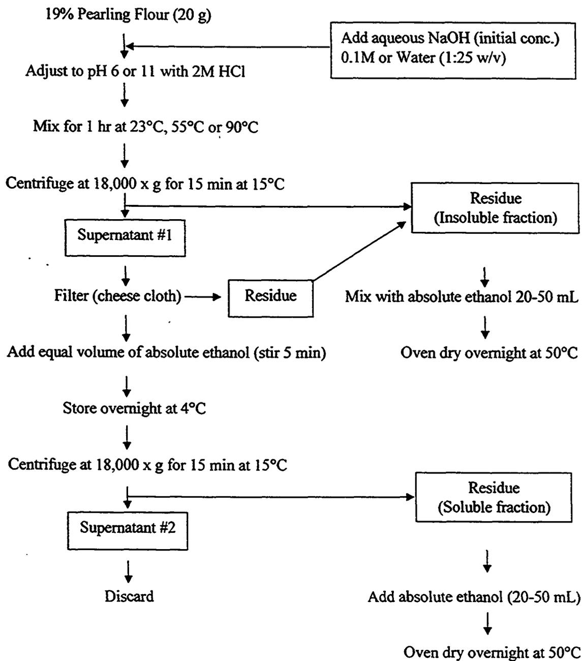
**Figure 3.2.** Flow diagram for the recovery of soluble and insoluble fractions from 19% pearling flour of CDC Candle barley at different temperatures.
