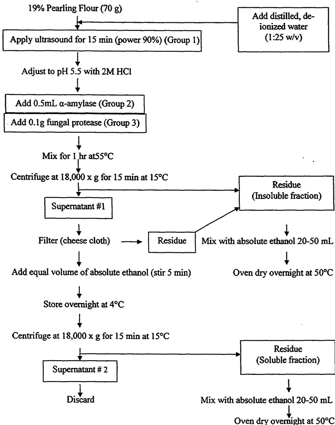
**Figure 4.1.** Flow diagram for the recovery of soluble and insoluble fractions from 19% pearling flour of CDC Candle barley using different enzymatic or ultrasound treatments.
