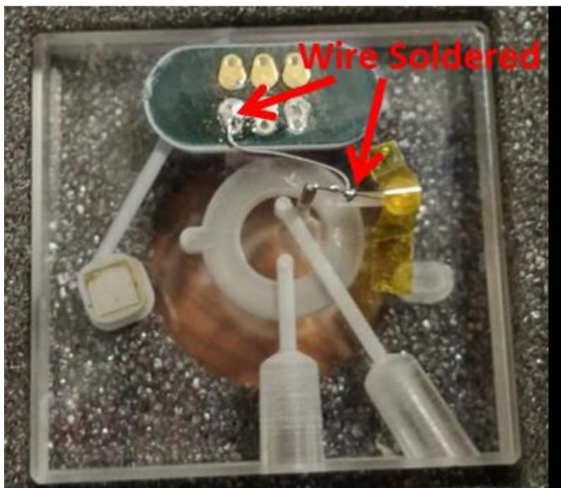
Fig. B1: Electrical connection between tip and the fluid AFM head by soldering a wire for KPFM analysis
