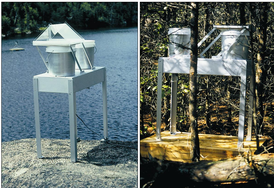
Figure 2.2 Automated wet deposition collectors (Aerochem Metrics) situated in the open (left panel) and under the forest canopy (upland jack pine; right panel) in the METAALICUS watershed.
