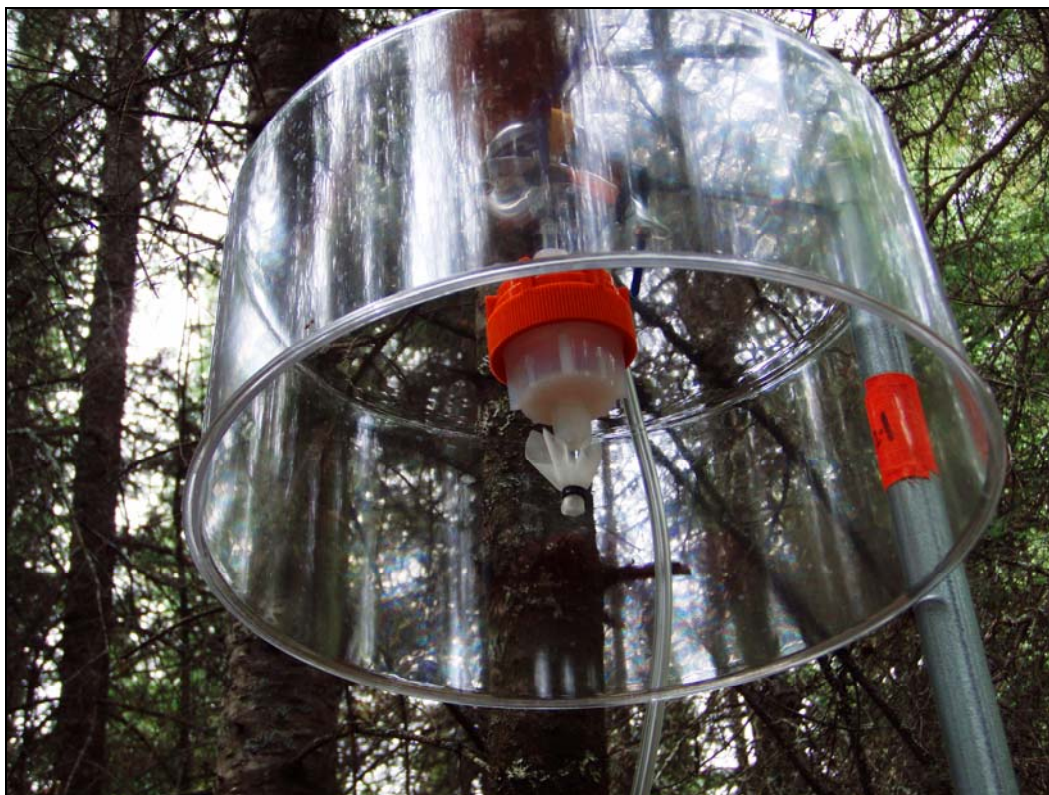
Figure 2.4 Example of p-MeHg sampling under the old growth canopy. Shown here is the sampling unit mounted 1.5 m above ground with the Teflon filter pack housing a QM-A filter capped with Nytex screening and sheltered under a plastic dome to prevent filters from being wetted during precipitation events. Tubing is connected to a constant flow high volume air sampling pump (SKC Inc., 224-PCXR8 Universal Sample Pump; not shown).
