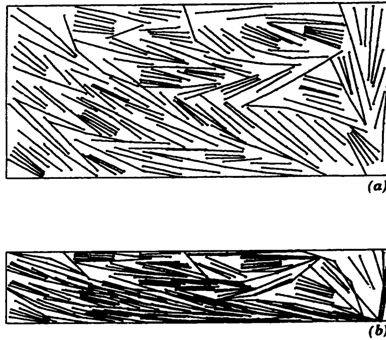
Figure 2.33 Distinct element method in consolidation (Anandarajah 1994); Distinct element assembly at two stages during one-dimensional compression: (a) void ratio e = 1.868 ; (b) void ratio e = 0.800
