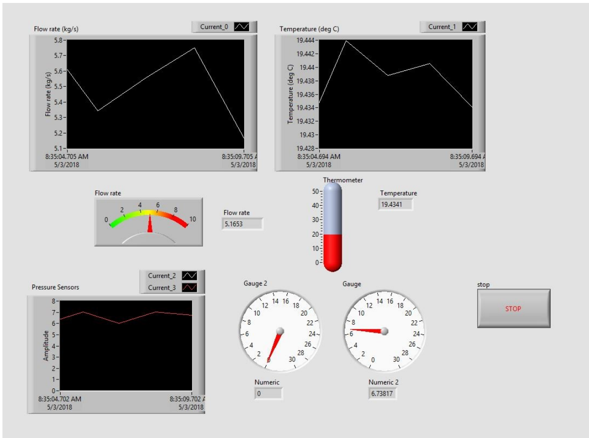
Figure 2.8. LabView block program (front interface)
