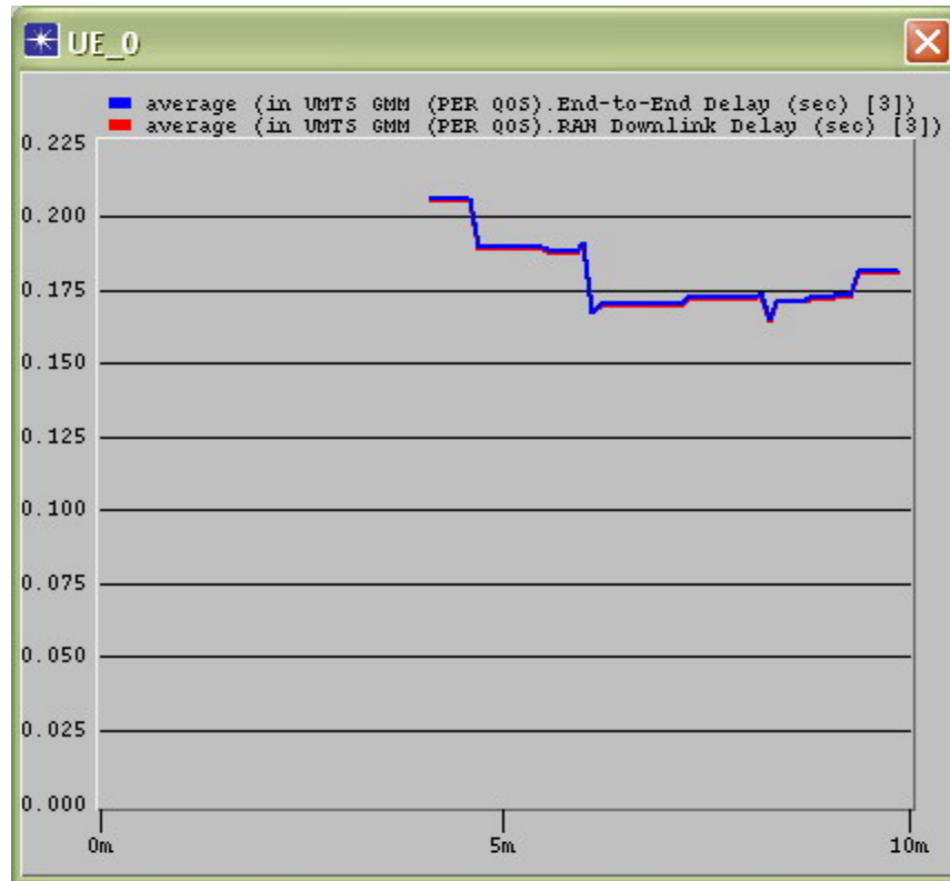
Figure 5-15 UE_0 (Per QoS) End-end end Delay (sec) and RAN DL Delay (sec)
