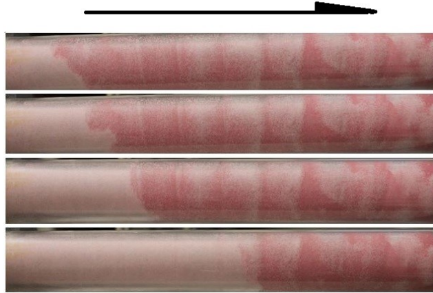
Figure 4.3.2. Foam propagation of surfactant-nanoparticle and surfactant-nanoparticle-polymer tests (the arrow showing as injection direction)
