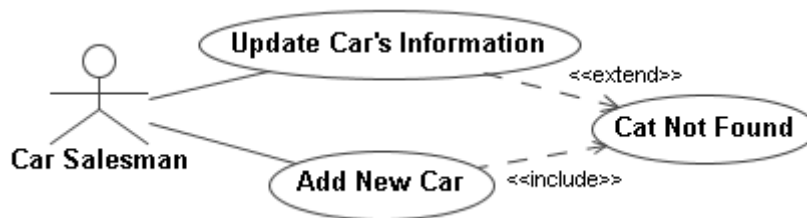
Figure 4-7: UC Car Not Found was incorrectly used for the purposes of containing common functionality and exception-handling behavior.
