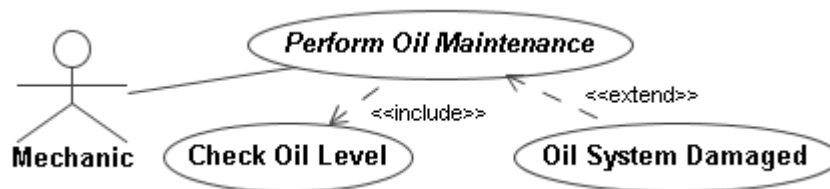
Figure 4-26: an abstract UC including subroutine behavior and being extended by a UC containing exceptional or optional behavior
