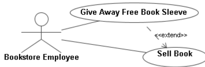
Figure 4-14: A good scenario of directly accessing an extending UC to allow independent initiation of an optional service
