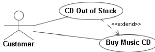
Figure 4-16: The actor is allowed to directly access the extension UC since the actor is the source of information required by the extension UC.
