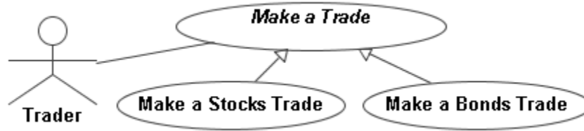
Figure 4-29: The abstract UC is associated with its specializing UCs using the generalization relationship
