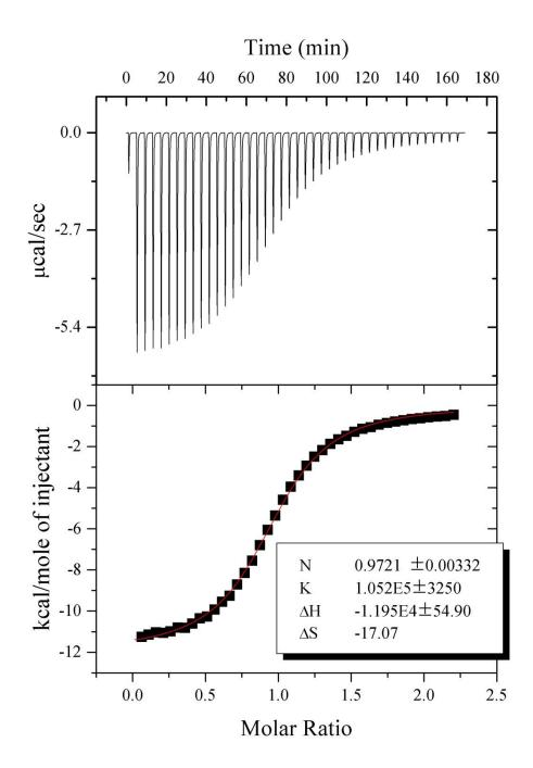
**Figure S3.** ITC data measured for the binding of Lyz (0.202 mM) to **L3** (2.0 mM) in aqueous ammonium acetate (50 mM, pH 6.8 and 25 °C) solutions.
