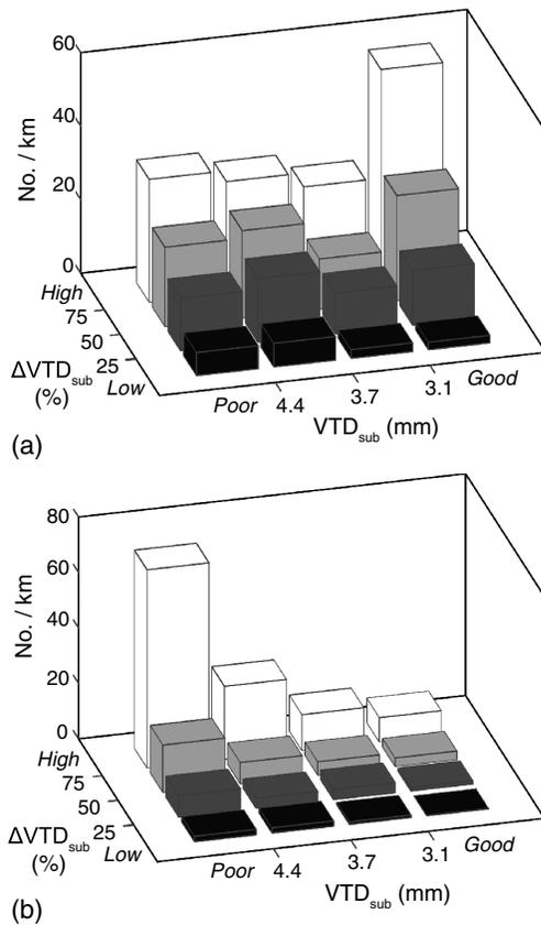
**Fig. 5.** Plots of the distribution of the number of Class 4: (a) gauge; (b) surface (warp, crosslevel, and profile) defects per km within the divisions of  $VTD_{sub}$  and  $\Delta VTD_{sub}$ ; these defects include both urgent and priority defects for both the subdivision in the Prairies and in the Canadian Shield
