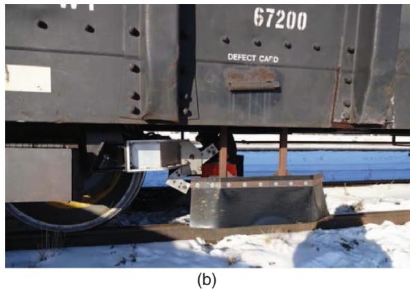
**Fig. 1.** (Color) (a) Configuration of the MRail system and the definition of VTD measurement (reprinted from Roghani and Hendry 2016, © ASCE); (b) photograph of the MRail system installed on a car used to collect the VTD measurements for this study (image by Alireza Roghani)
