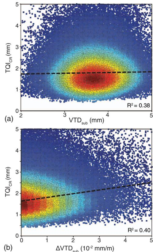
**Fig. 10.** (Color) Plots of  $TQI_{CR}$  versus (a)  $VTD_{sub}$ ; (b)  $\Delta VTD_{sub}$ ; the color denotes the density of the data points, with the highest density shown in red; the colors are intended to be a qualitative representation and thus a legend is not provided; the dashed lines are the linear fits to the data presented for discussion
