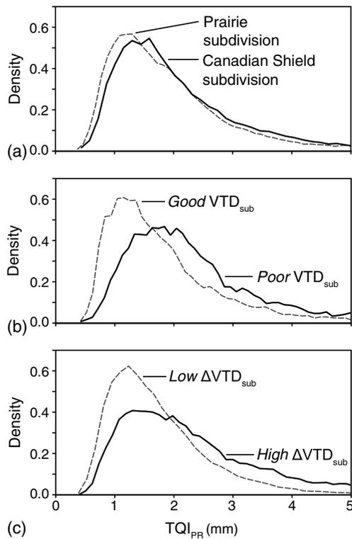
**Fig. 11.** Plots comparing the distribution of (a) the  $TQI_{PR}$  for the Prairie and the Canadian Shield subdivisions; (b) the  $TQI_{PR}$  for track divided into subsets of good and poor  $VTD_{sub}$ ; (c) the  $TQI_{PR}$  for track divided into subsets of high and low  $\Delta VTD_{sub}$ , where good  $VTD_{sub}$  is  $<3.1$  mm, poor  $VTD_{sub}$  is  $>4.4$  mm, low  $\Delta VTD_{sub}$  is  $<0.003$  mm/m, and high  $\Delta VTD_{sub}$  is  $>0.013$  mm/m
