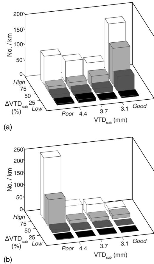
**Fig. 6.** Plots of the distribution of the number of Class 3: (a) gauge; (b) surface (warp, crosslevel, and profile) defects per km within the divisions of  $VTD_{sub}$  and  $\Delta VTD_{sub}$ ; these defects include both urgent and priority defects for both the subdivision in the Prairies and in the Canadian Shield
