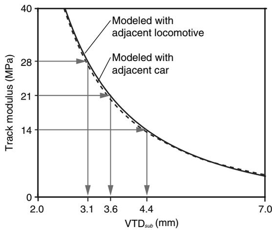
**Fig. 2.** Plot showing the modeled relationship between  $VTD_{sub}$  and track modulus for the two loading conditions under which measurements were obtained; note: the Prairies subdivision measurements were taken with a locomotive adjacent to the MRail system and the Canadian Shield with a loaded rail car adjacent to the MRail system
