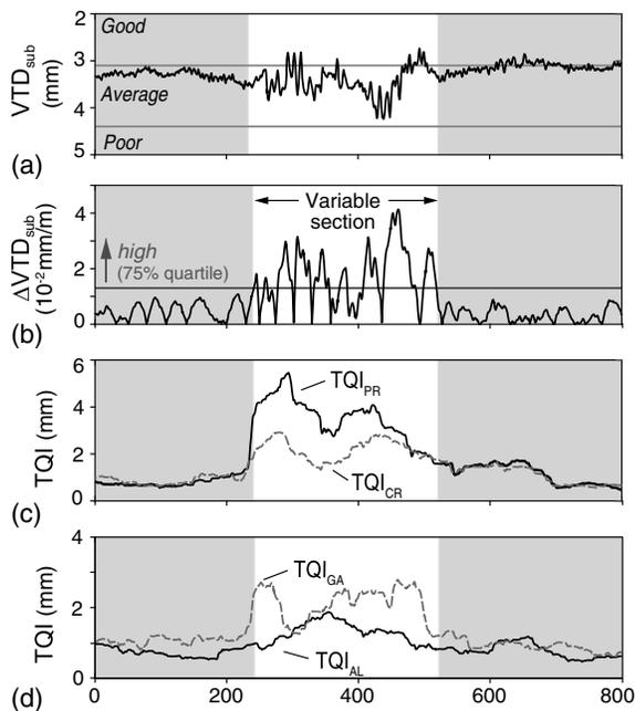
**Fig. 9.** Plots of the (a)  $VTD_{sub}$ ; (b)  $\Delta VTD_{sub}$ ; (c)  $TQI_{PR}$  and  $TQI_{CR}$ ; (d)  $TQI_{GA}$  and  $TQI_{AL}$  for an 800-m section of track of average to good track conditions (based on  $VTD_{sub}$ , with a 270-m section of track with elevated  $\Delta VTD_{sub}$ )
