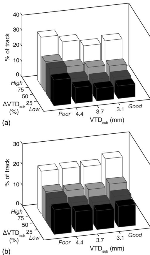
**Fig. 13.** Plots of the percentage of total length of track with (a)  $TQI_{GA} > 3$  mm; (b) surface-related  $TQI > 3$  mm within the divisions of  $VTD_{sub}$  and  $\Delta VTD_{sub}$ ; these plots include data from both the subdivision in the Prairies and the subdivision in the Canadian Shield
