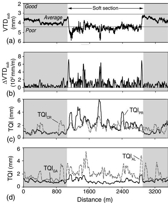
**Fig. 8.** Plots of the (a)  $VTD_{sub}$ ; (b)  $\Delta VTD_{sub}$ ; (c)  $TQI_{PR}$  and  $TQI_{CR}$ ; (d)  $TQI_{GA}$  and  $TQI_{AL}$  for a 2-km example of poor track conditions
