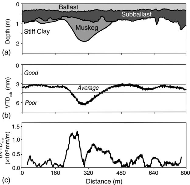
**Fig. 4.** Example over an 800-m section of track with a section of soft muskeg subgrade to demonstrate the resulting VTD metrics, where (a) the composition of track substructure and the location of a soft muskeg section; (b) the  $VTD_{sub}$  (data from Roghani and Hendry 2016); (c) the  $\Delta VTD_{sub}$
