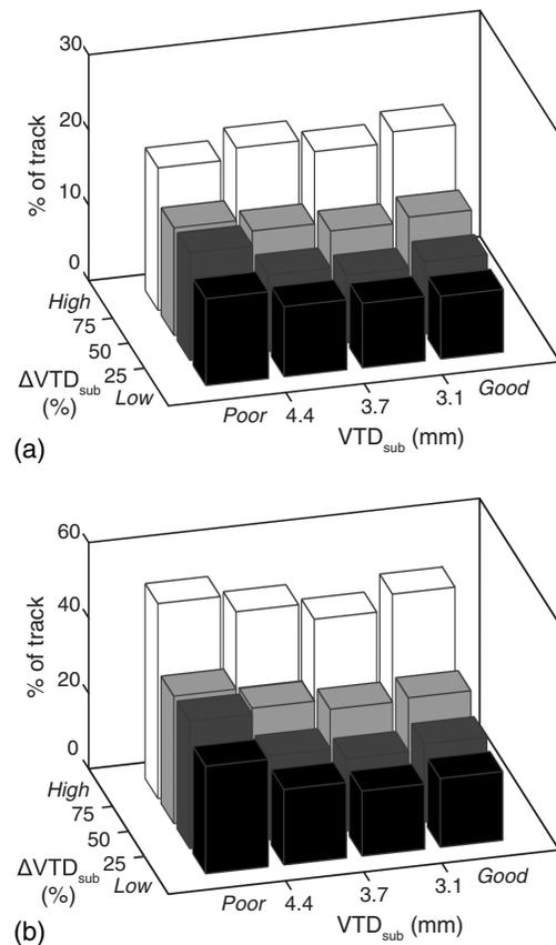
**Fig. 12.** Plots of the percentage of total length of track with (a)  $TQI_{GA} > 3$  mm; (b) surface-related TQI  $> 3$  mm within the divisions of  $VTD_{sub}$  and  $\Delta VTD_{sub}$ ; these plots include data from both the subdivision in the Prairies and the subdivision in the Canadian Shield
