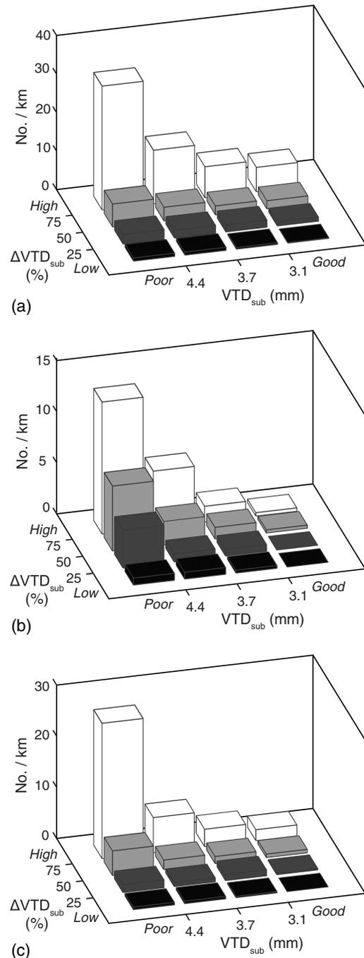
**Fig. 7.** Plots of the distribution of the combined number of Class 4 surface defects per km divided into (a) warp; (b) crosslevel; (c) profile defects within the divisions of  $VTD_{sub}$  and  $\Delta VTD_{sub}$ ; these defects include both urgent and priority defects for both the subdivision in the Prairies and in the Canadian Shield
