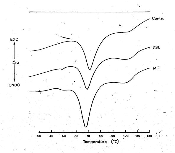
Figure 4.11 DSC thermograms of batters (heating rate 10 C°/min).
