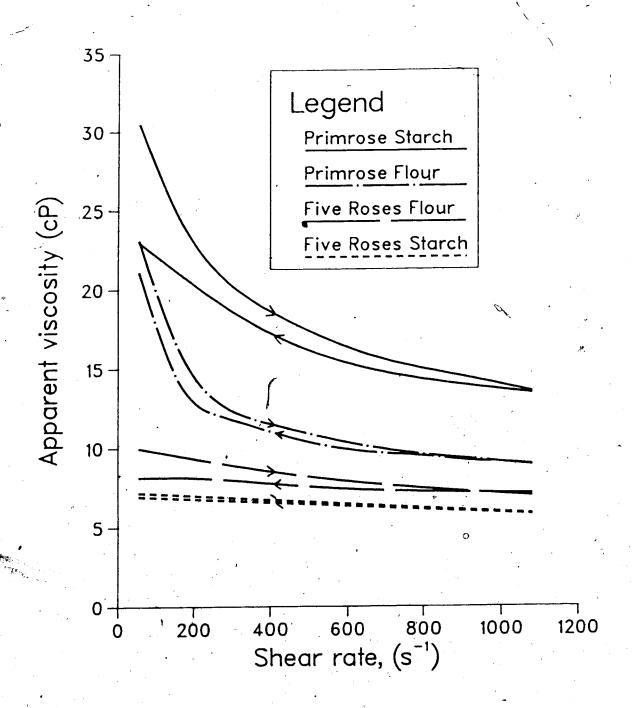
Figure 4.5 Viscosity of starches and flours.
