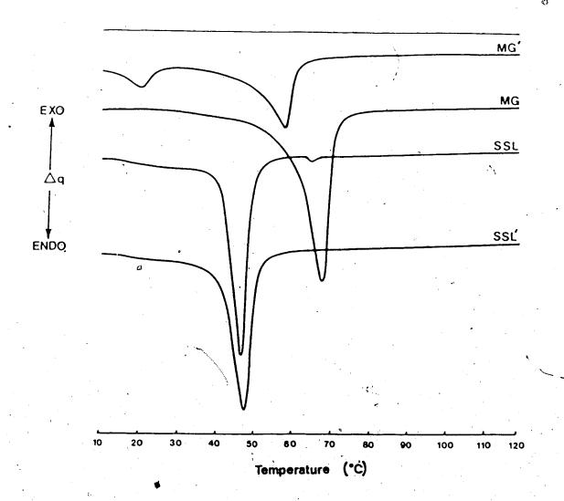
Figure 4.7 DSC thermograms of emulsifiers. MG; MG (MG reheated); SSL; SSL' (SSL reheated).
