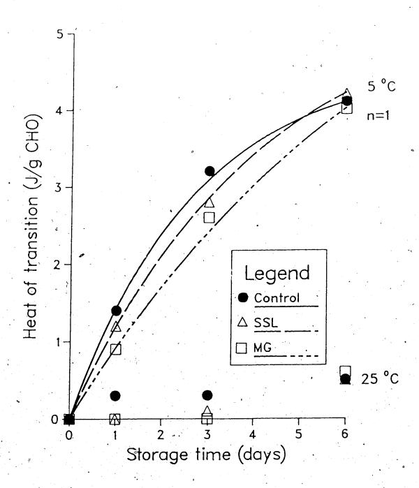
Figure 4.14 Staling endotherm data of storage trial II. Avrami model, n=1 at 5°C.
