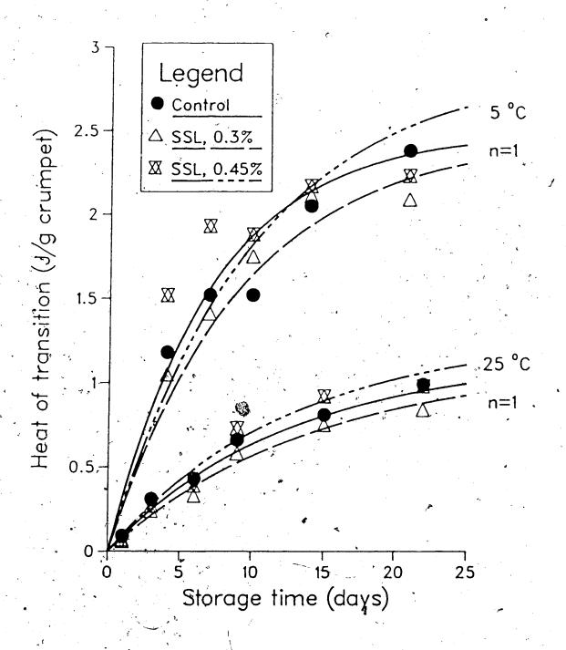
Figure 4.23 Staling endotherm data of storage Trial IV. Avrami models, n=1 at 5 and 25°C.
