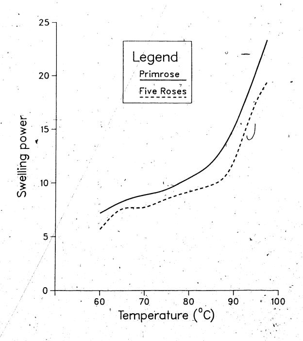
Figure 4.1 Swelling power of the starches as a function of temperature.
