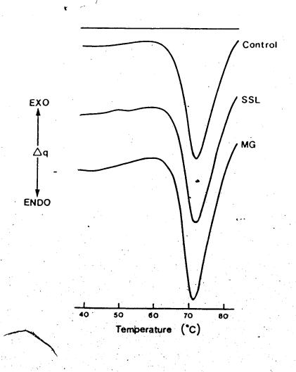
Figure 4.10 DSC thermograms of batter during "cooking" regime (heating rate 20 C°/min).
