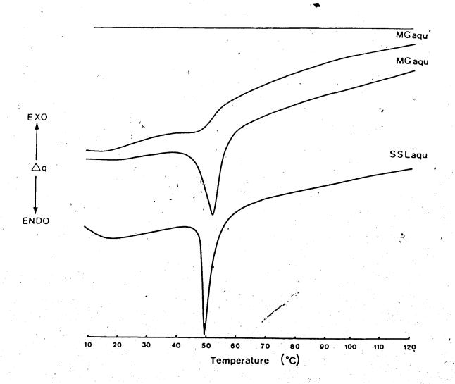
Figure 4.8 DSC thermograms of emulsifiers in presence of water. MGaqu; MGaqu' (MGaqu reheated); SSLaqu (SSLaqu reheated was unchanged).
