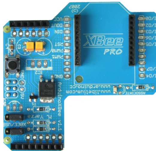
Fig 2.4 XBee Shield hardware specification
