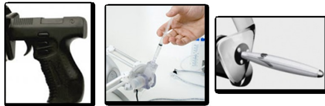
Figure 3-2 The Falcon alternative user interfaces: pistol grip (left), needle insertion (middle), and a pen-shaped stylus (right)
