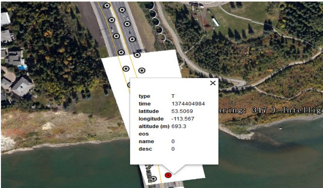
Figure 20 Location information for first point entering Geofence
