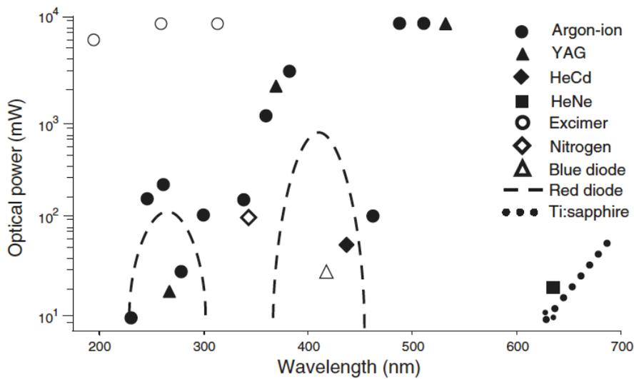
**Figure 1.5** Output power and wavelengths of various laser systems used in LIF detection. Reprinted from Ref. [41] with permission from Elsevier.
