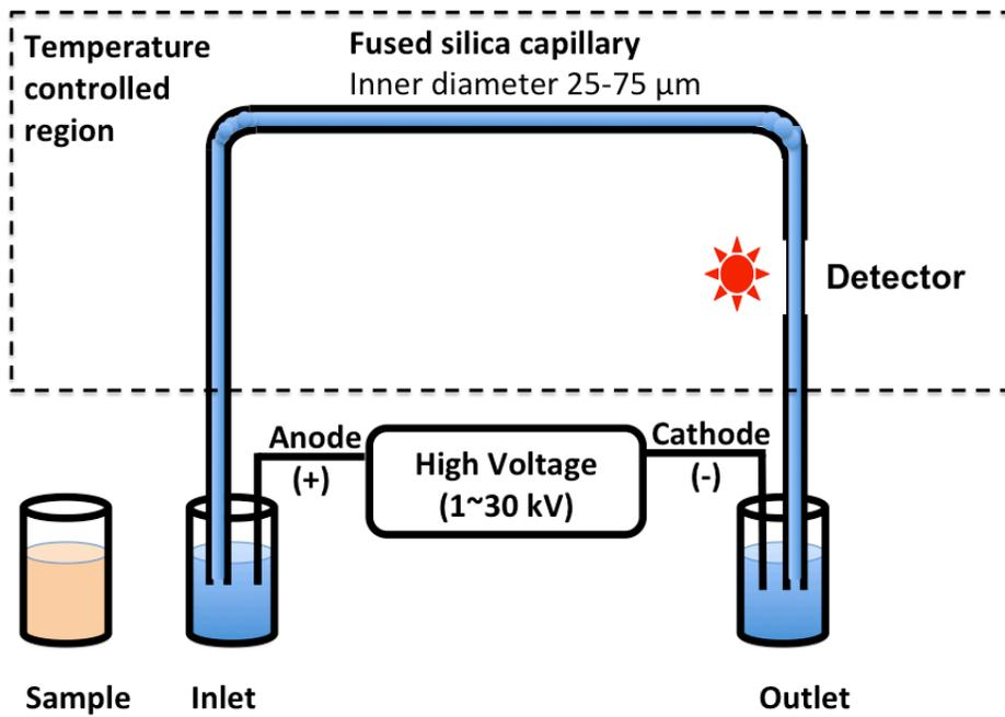
Figure 1.1 A schematic setup for capillary electrophoresis instrument
