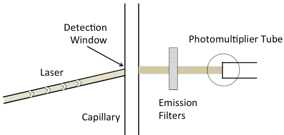
**Figure 1.4** Schematic diagram of the optical setup of the Beckman PA 800 plus LIF detection system. Adapted from Beckman PA 800 plus manual.
