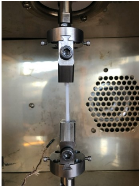
Figure 3.7 Tensile testing of POM filament
