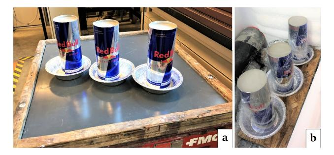
Figure 3-11 Filling the mud molds on the vibrating table (a) Mud samples inside the freezer (b)
