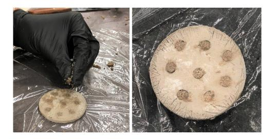
Figure 3-21 Sand filling of a penetrated mud layer
