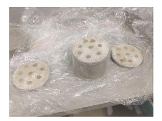
Figure 3-23 Staking IHS mud layer for bioturbated sample
