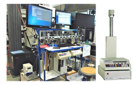
Figure 3-30 ISCO® 260D syringe pump (Teledyne ISCO®, 2017)
