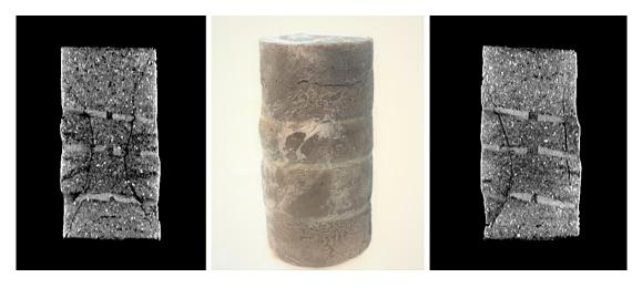
Figure 6-11 Bioturbated IHS sample loaded in an isotropically consolidated drained shear test under  $\sigma_3$  of 0.5 MPa
