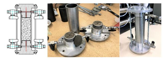
Figure 3-6 Sand packing assembly
