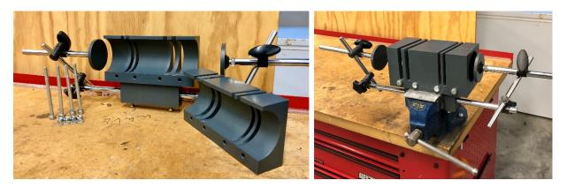
Figure 3-17 Mudstone cutter box (63.5 millimeters diameter)
