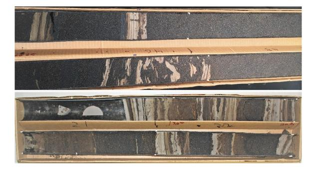
Figure 3-27 McMurray Formation half-cut IHS cores
