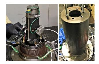
Figure 3-32 Triaxial Cell
