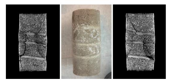
Figure 6-10 IHS sample loaded in an isotropically consolidated drained shear test under  $\sigma_3$  of 0.5 MPa
