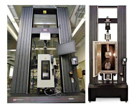
Figure 3-31 INSTRON® 5988 Floor Model testing system (Instron®, 2017)
