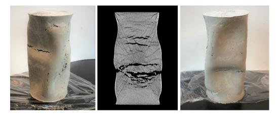
Figure 5-10 Mud sample loaded in an isotropically consolidated drained shear test under  $\sigma_3$  of 0.5 MPa
