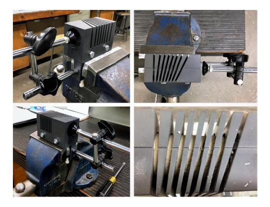
Figure 3-16 Mudstone cutter box (38.1 millimeters diameter)
