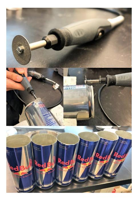
Figure 3-10 Mud samples' mold preparation using a Dremel rotary cutter
