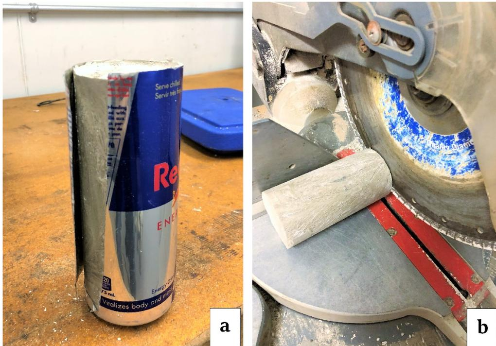
Figure 3-12 Cutting the mold using a cutter (a), Trimming a frozen mud sample using a masonry saw (b)
