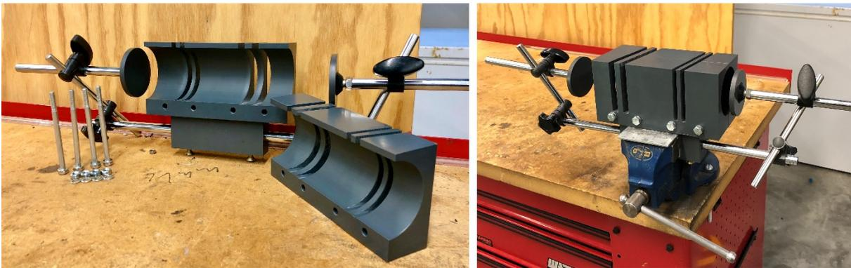
Figure 3-17 Mudstone cutter box (63.5 millimeters diameter)
