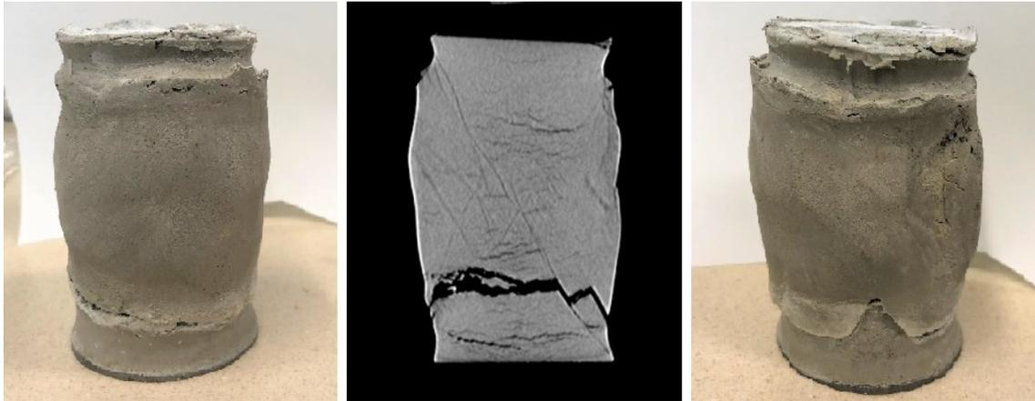
Figure 5-8 Mud sample loaded in an isotropically consolidated drained shear test under  $\sigma_3'$  of 3.5 MPa
