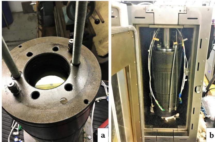
Figure 3-24 Consolidation of analog IHS sample
