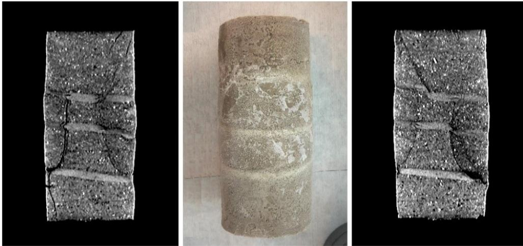
Figure 6-10 IHS sample loaded in an isotropically consolidated drained shear test under  $\sigma_3'$  of 0.5 MPa
