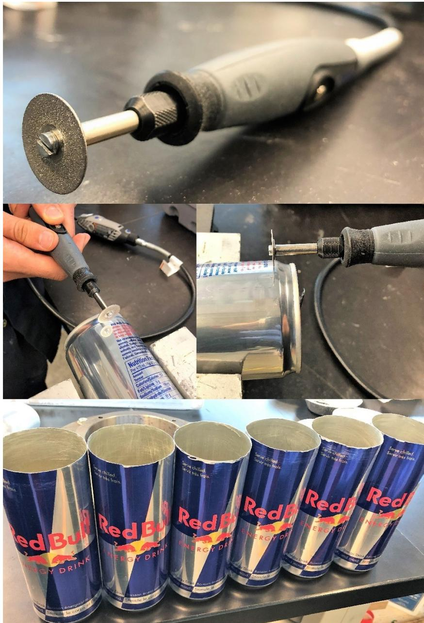
Figure 3-10 Mud samples' mold preparation using a Dremel rotary cutter
