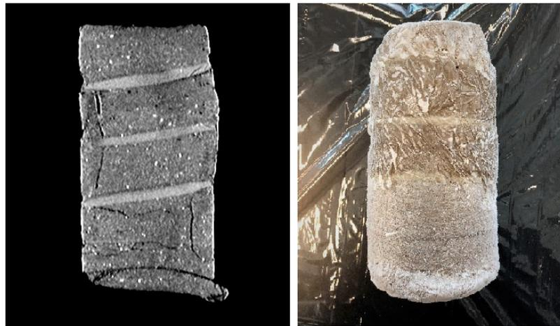
Figure 6-8 IHS sample loaded in an isotropically consolidated drained shear test under  $\sigma_3'$  of 3.5 MPa
