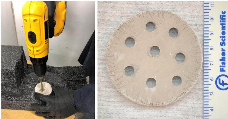
Figure 3-20 Penetrating a mud layer using a power drill
