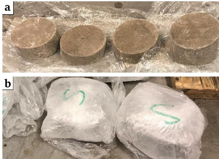
Figure 3-15 Sliced analog sand sample (a), Wrapped sand slices (b)
