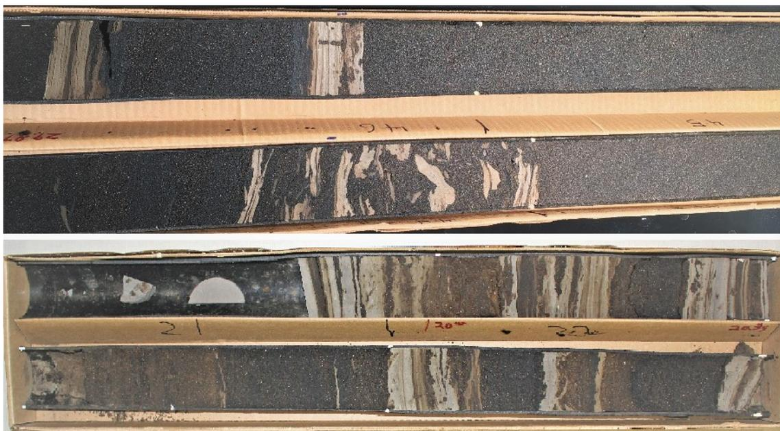
Figure 3-27 McMurray Formation half-cut IHS cores
