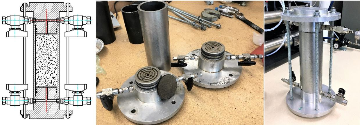
Figure 3-6 Sand packing assembly
