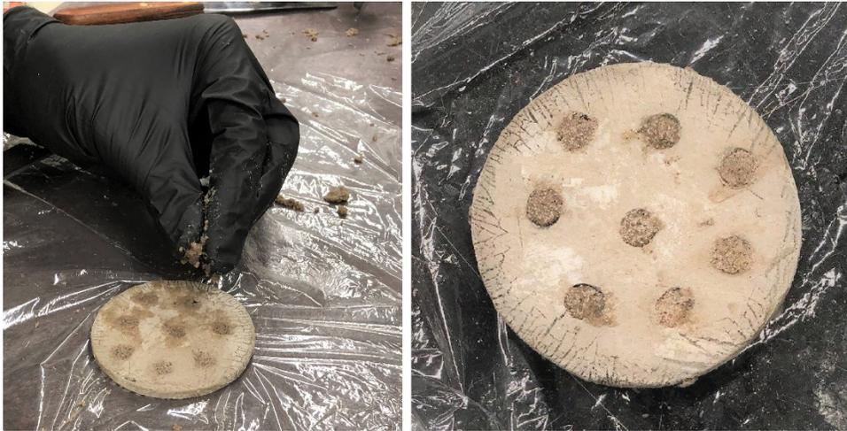
Figure 3-21 Sand filling of a penetrated mud layer
