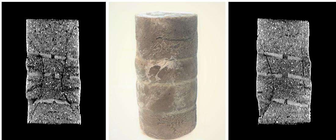
Figure 6-11 Bioturbated IHS sample loaded in an isotropically consolidated drained shear test under  $\sigma_3'$  of 0.5 MPa
