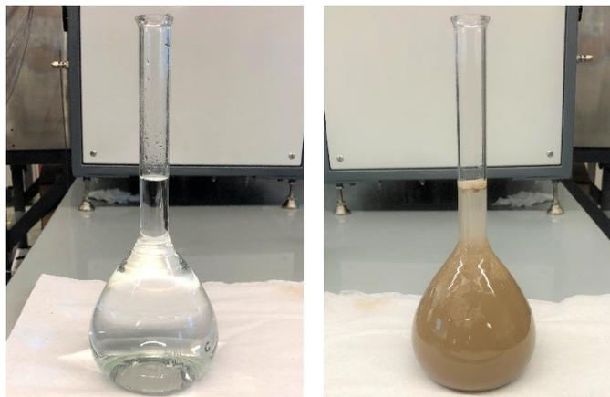
Figure 3-2 Volumetric flask filled with water (left) and sand-water mixture (right)
