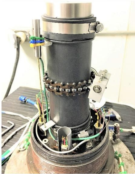
Figure 3-8 Preparation of analog sand sample for hydro-mechanical testing
