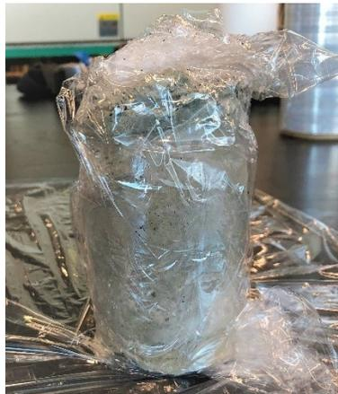
Figure 5-9 Mud sample loaded in an isotropically consolidated drained shear test under  $\sigma_3'$  of 1 MPa
