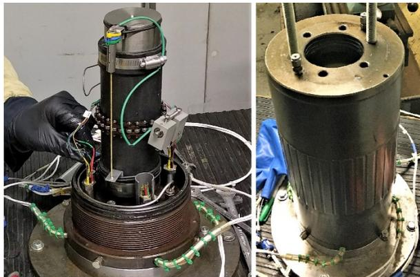
Figure 3-32 Triaxial Cell
