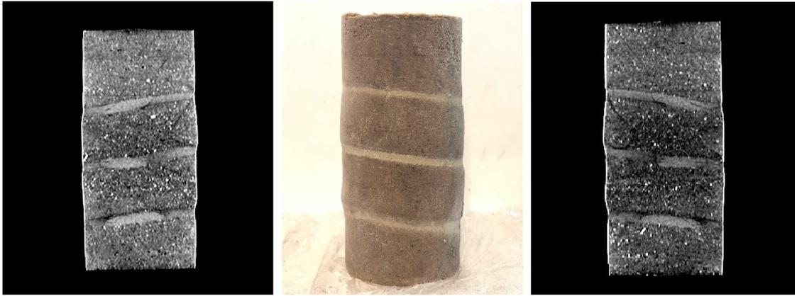
Figure 6-9 IHS sample loaded in an isotropically consolidated drained shear test under  $\sigma_3'$  of 1 MPa
