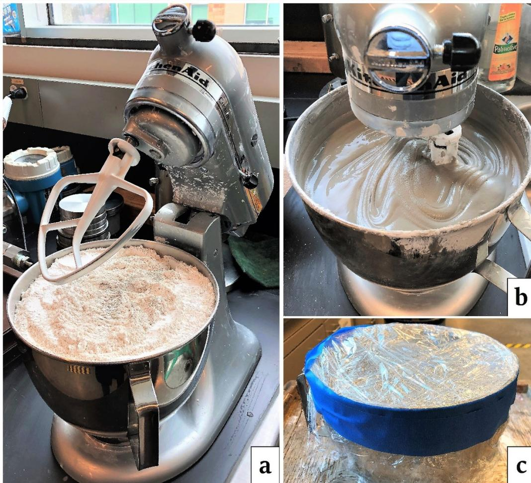
Figure 3-9 Silt and kaolinite mixture (a), Silt-kaolinite slurry (b), Soaking stage (c)
