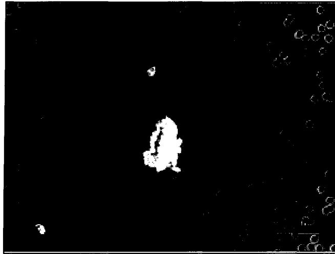
Figure 4-26 SEM micrograph showing a large particle detected on a 10 \mu\text{m} PCTE membrane filter (Magn. = 200x).
