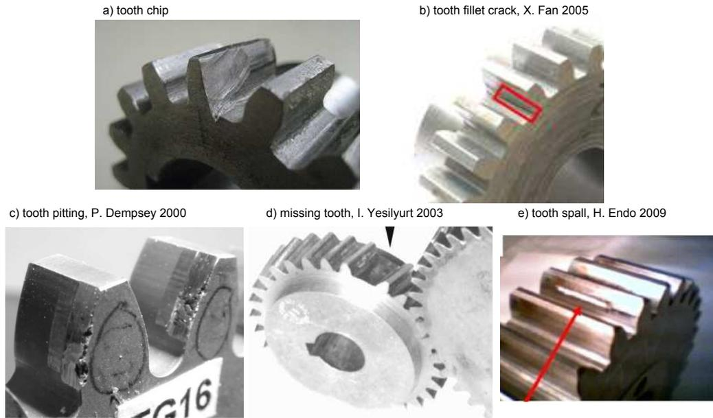
Figure 2.1: Example gear faults under a) tooth chip, b) tooth fillet crack [11], c) tooth pitting [12], d) missing tooth [13], and e) tooth spall [14] cases.
