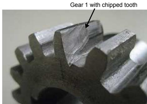
Figure 4.7: Faulty gear 1 with seeded tooth chip.
