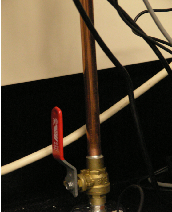
Figure A- 1. Compressed air line connected to the rheometer
