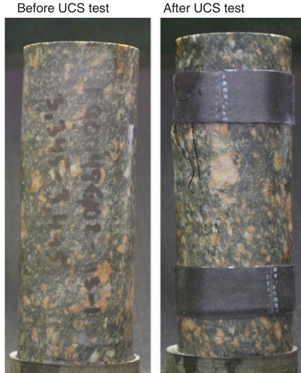
**Figure 3.12: Sample of Äspö Diorite used to compare the crack-initiation stress using various methods. The specimen is mostly composed of Plagioclase, Oligoclase (in orange) and Anorthite (dark brown). Quartz grains are rarely observable as light coloured mineral while K-feldspars are not obvious in the specimen.**
