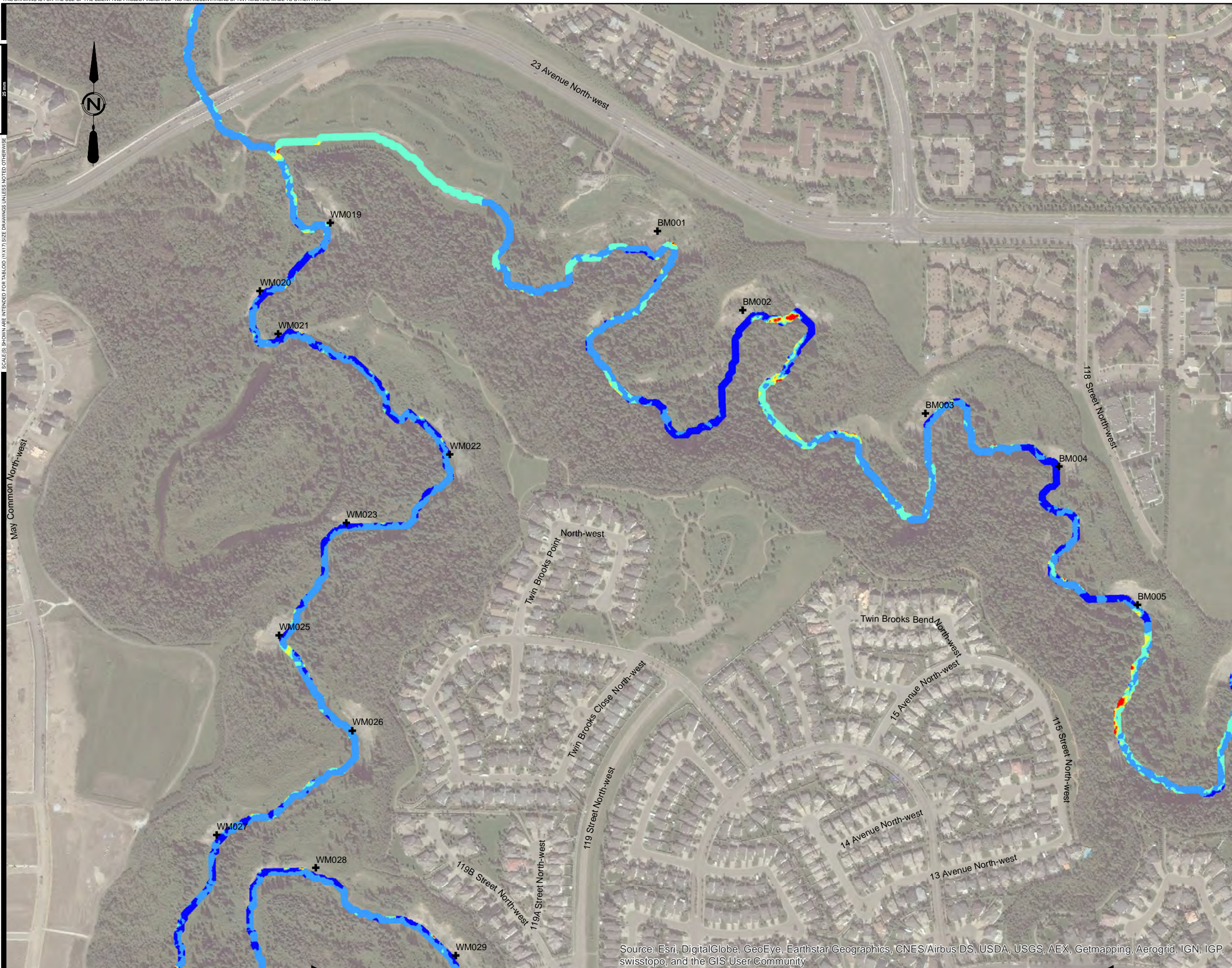
FIGURE No. 2-12 BLACKMUD/WHITEMUD CREEK WATERSHED MANAGEMENT STUDY FUTURE DEVELOPMENT DISCHARGE RATE 5.0 L/s/ha RATIO TO EXISTING - 100 YEAR FLOOD VELOCITY AE PROJECT No. 2016-3785 SCALE 1:5,000 APPROVED DATE 2017 MARCH REV DESCRIPTION ISSUED FOR REPORT
