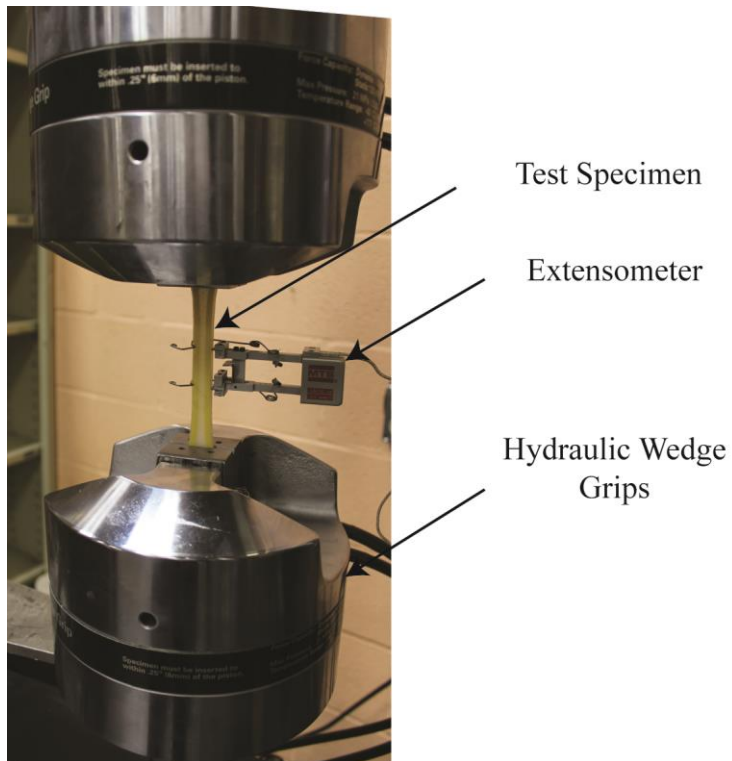
Figure 3: Mechanical testing setup to evaluate the tensile properties of Kevlar reinforced 3D printed specimen
