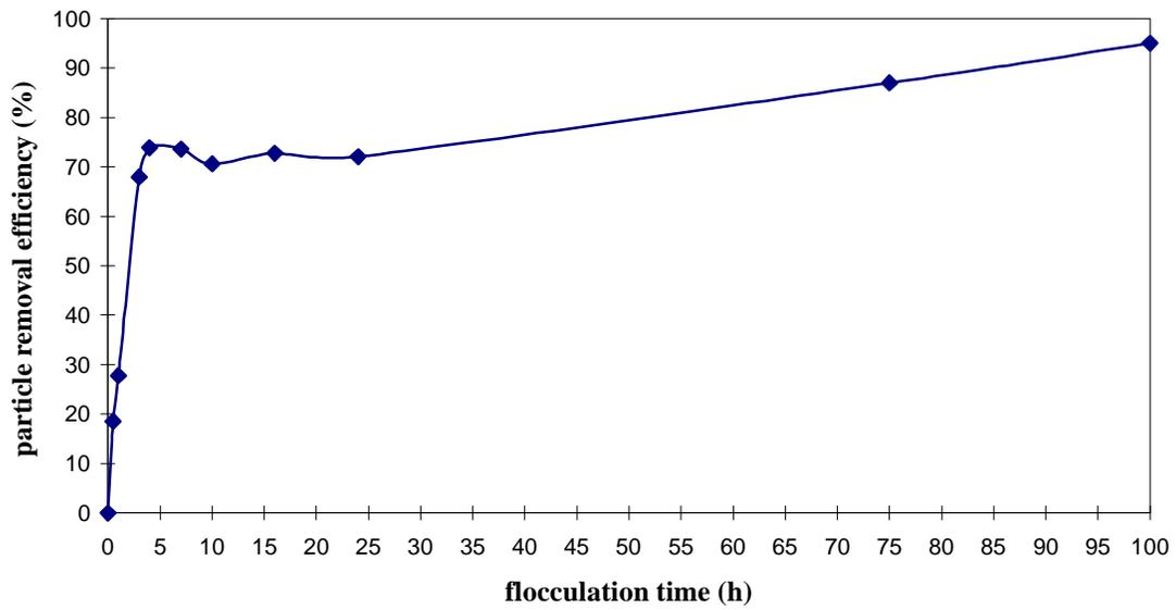
**Figure 5:** Effect of flocculation time on the particle removal efficiency of mixtures of pulp mill effluent and river water ( $V_{WHPME} : V_{ARW} = 1:1$ , sampling date: Aug. 19, 1998,  $V_{GS} = 2$  mm/s)
