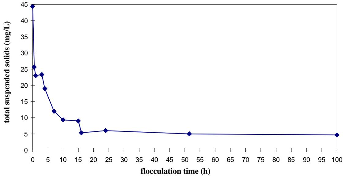
**Figure 7:** Effect of flocculation time on the total suspended solids of mixtures of pulp mill effluent and river water ( $V_{\text{WHPME}} : V_{\text{ARW}} = 1:1$ , sampling date: Aug. 19, 1998,  $V_{\text{GS}} = 2 \text{ mm/s}$ )
