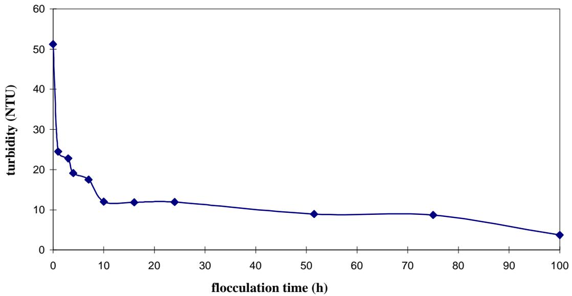
**Figure 6:** Effect of flocculation time on the turbidity of mixtures of pulp mill effluent and river water ( $V_{WHPME} : V_{ARW} = 1:1$ , sampling date: Aug. 19, 1998,  $V_{GS} = 2$  mm/s)
