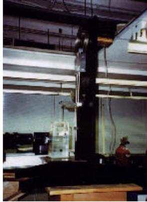
**Figure 3:** A vertically oscillating-grid mixing system
