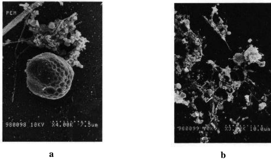
**Figure 8:** Flocs formed from a mixture of PME and river water with a volume ratio of 1:1
