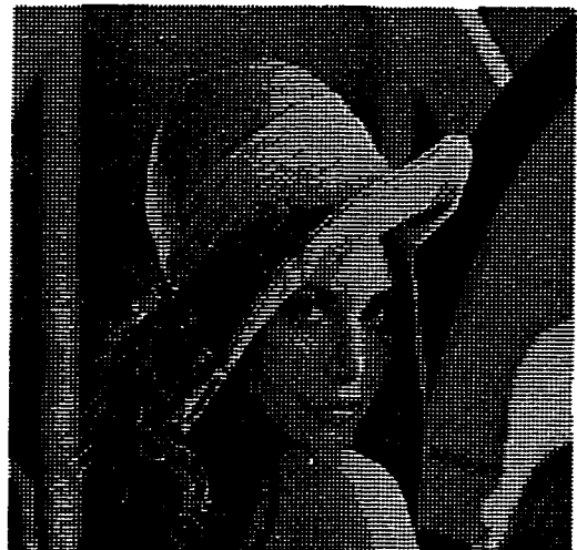
Figure 5.2: Threshold Matrix Clustered Ordered Dither using a 4x4 threshold matrix as shown in section 5.2.1.
