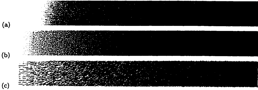
Figure 3.2: From top to bottom: (a) Original grey-scale image - 600dpi; (b) Importance Driven Halftoning using single pixel as display primitive - 200dpi; (c) Importance Driven Halftoning using a line segment oriented and scaled as a function of intensity - 200dpi. Both images in (b) and (c) set approximately 70,000 black pixels
