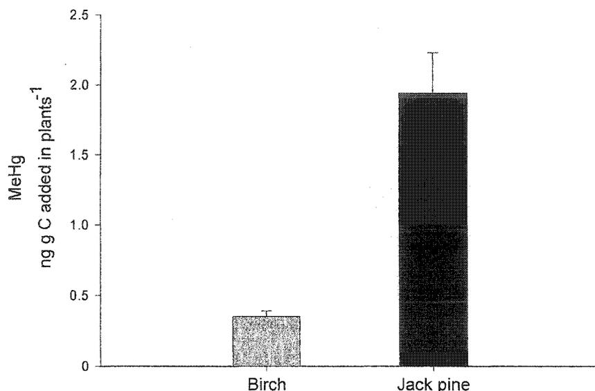
Figure 2-6. Net mass of methylmercury (MeHg) produced per mass of carbon added as either jack pine needles or birch leaves. Net MeHg production was calculated dividing net MeHg increases (Table 2-3) by the mass of C in dried plants at the beginning of the experiment (Table 2-1). MeHg production per g C added was calculated for each enclosure and then averaged.
