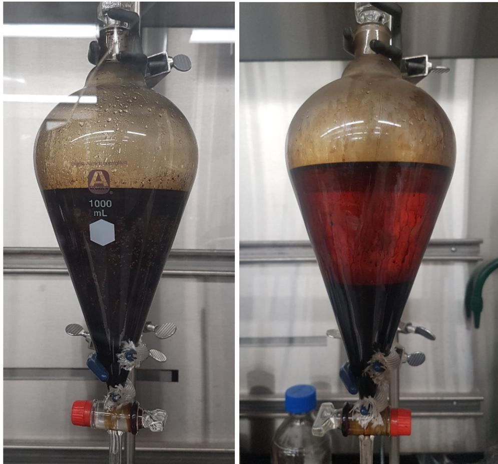
Figure 4.3 Conical separating funnel: (a) At the end of experiment, (b) After 24 hours into separation
