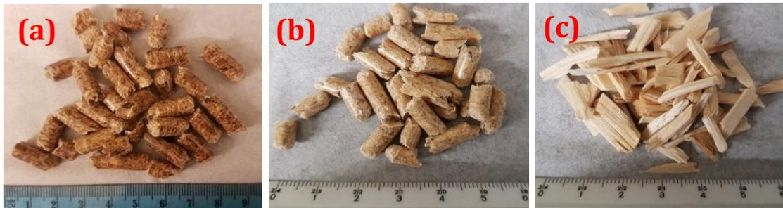
Figure 4.1 Feedstock: (a) Hardwood Pellets, (b) Softwood Pellets, (c) Softwood Chips
