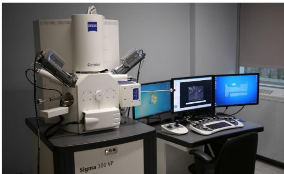
Figure 4.7 Scanning Electron Microscope Zeiss Sigma 300 VP-FESEM
