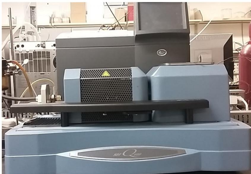
Figure 3.2 Thermogravimetric analyzer SDT Q600, TA Instruments
