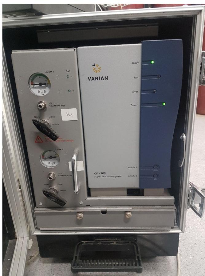
Figure 4.6 CP-4900 Micro Gas Chromatograph used for gas analysis
