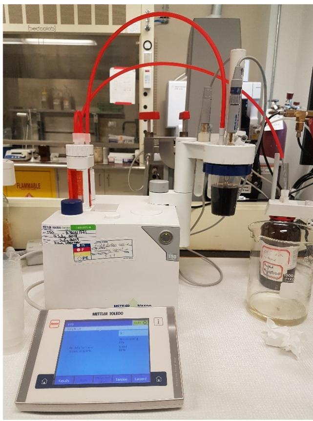
Figure 4.4 Mettler Toledo T50 for TAN measurement
