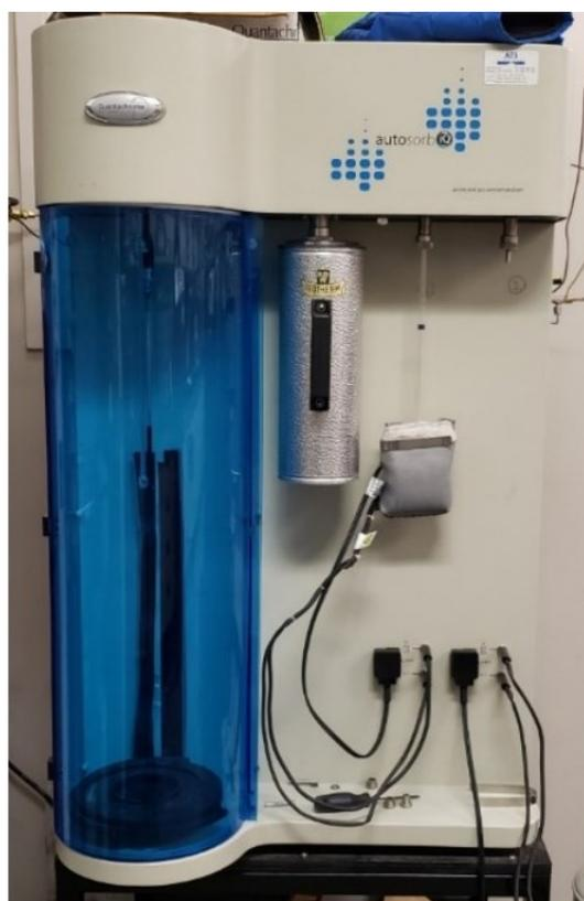
Figure 4.8 BET set-up, Quantachrome IQ
