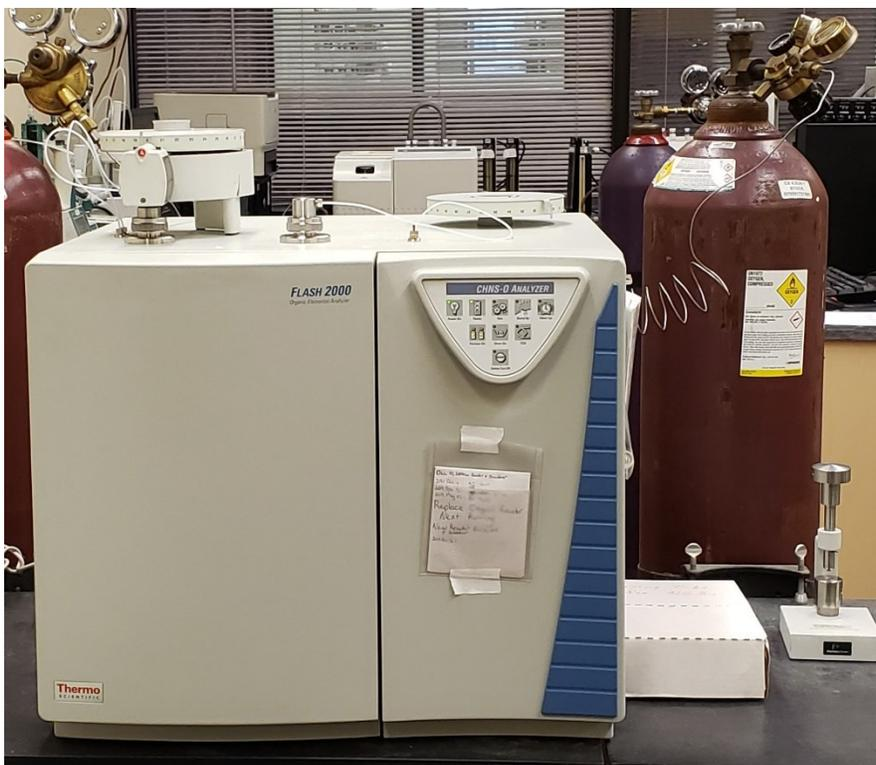
Figure 3.3 CHNS Analyzer
