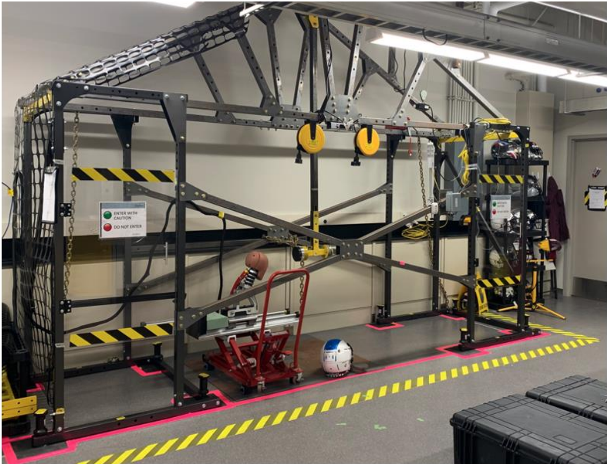
Figure 3.4: Pendulum impactor system, showing the steel pendulum arm with an MEP pad and steel plates. The Hybrid III head-neck assembly is located atop a translating linear rail. Reproduced with permission from Springer Nature, MacGillivray et al. [142] copyright 2021.
