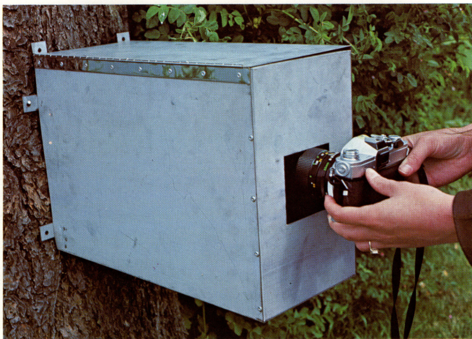
Figure 1. This sheet-metal shadow box provided uniform lighting (by flash) for lichen photographs. Circular metal tag used for all sites and quadrats is visible at top of open shadow box.
