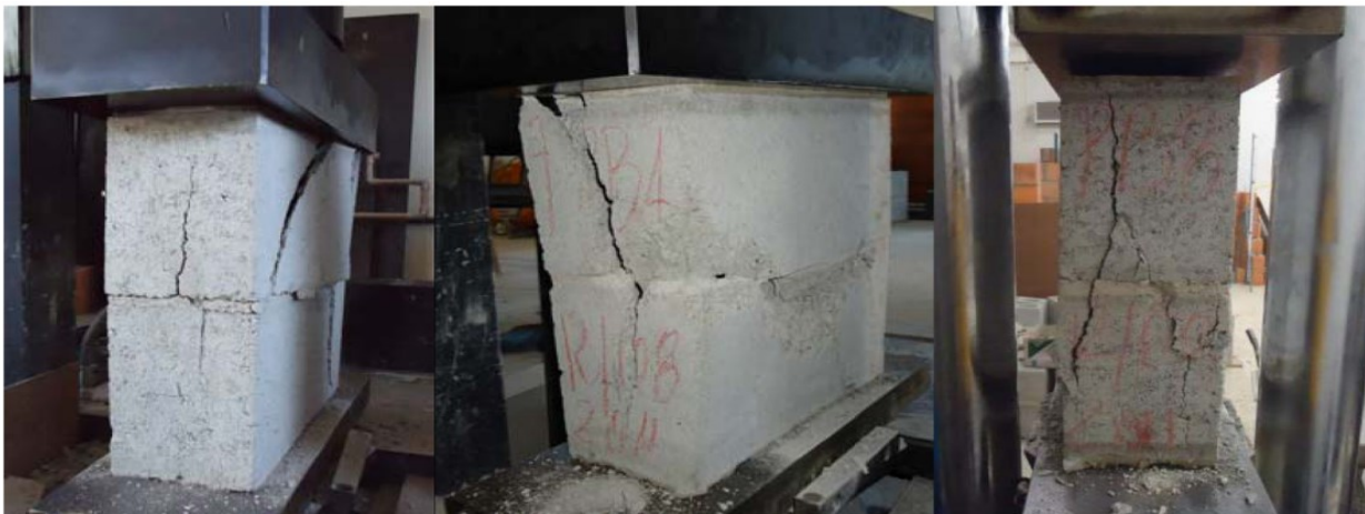
Figure 2-1: Capped masonry prism and failure of masonry prisms (Fortes et al. 2015)
